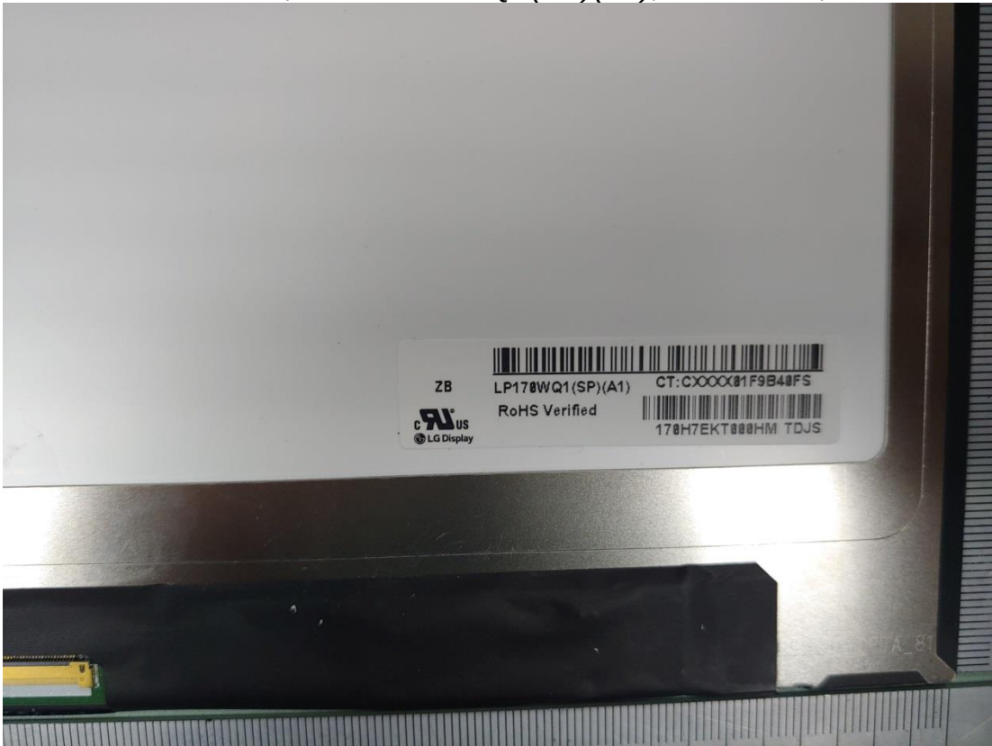
Figure 57 LGD, M/N LP170WQ1(SP)(A1), LCD Panel, Label View
