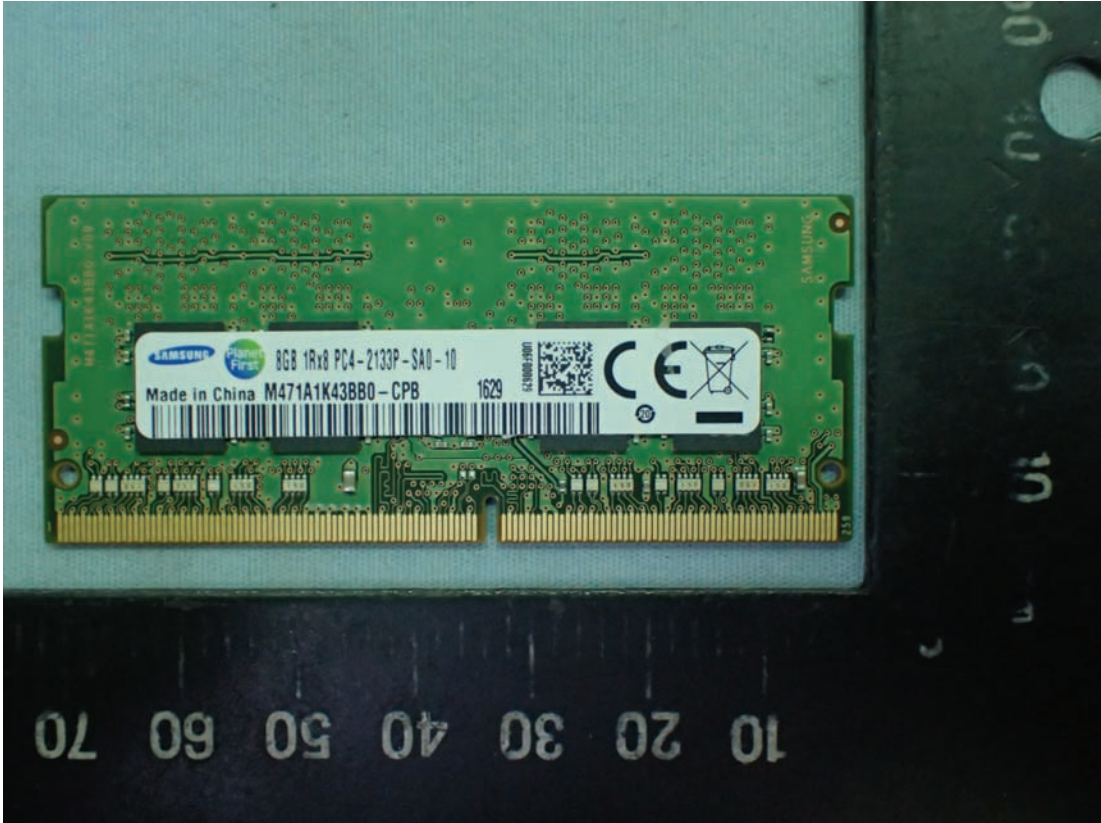
Figure 20 Internal View (SAMSUNG, M/N M471A1K43BB0-CPB Memory)
