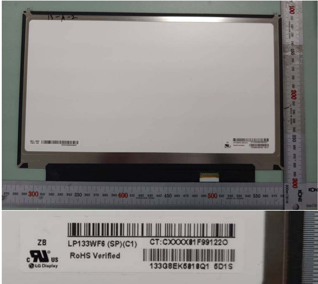
Figure 22 M/N: LP133WF6(SP)(C1)/(AIT Including touch), LCD Panel, Back/Label View
