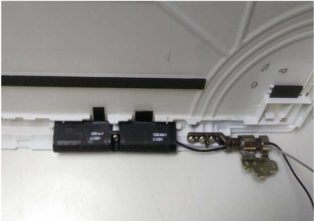
Figure 36 WLAN Combo Antenna Location
