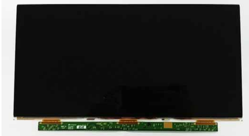
Figure 24 LG Display, M/N: LP133WF6(SP)(C1)/(AIT Including touch), LCD Panel, Front View
