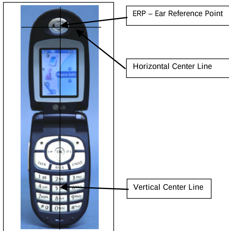
Figure 13.1 Handset Reference Points
