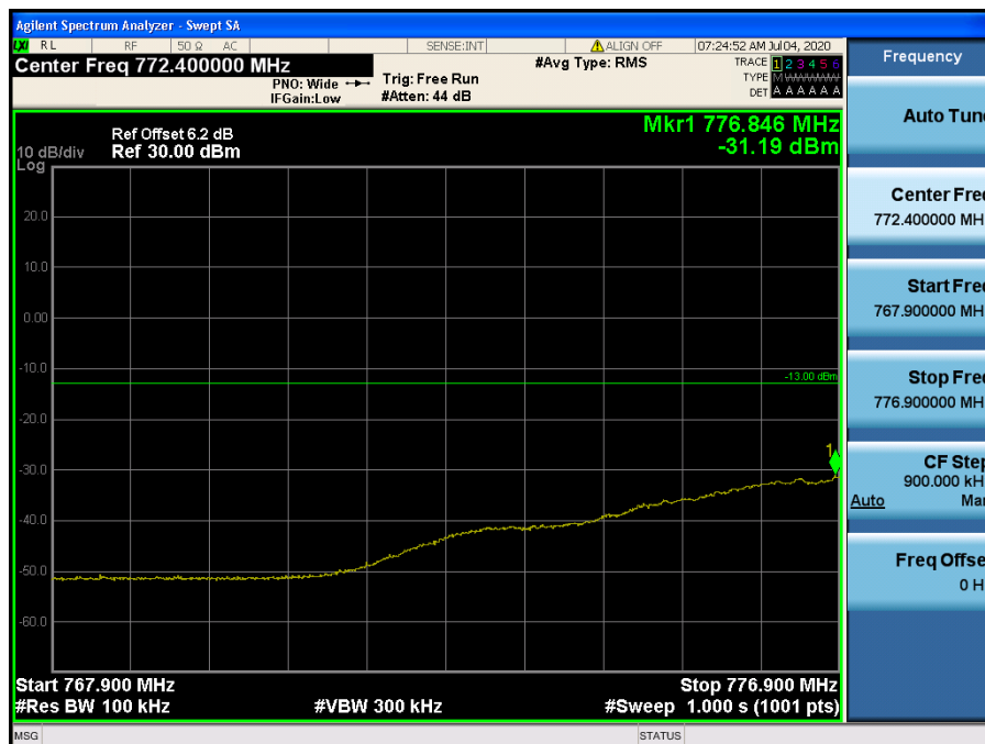
LTE Band 13 / 10MHz / QPSK - RB Size/Offset (50/0)
