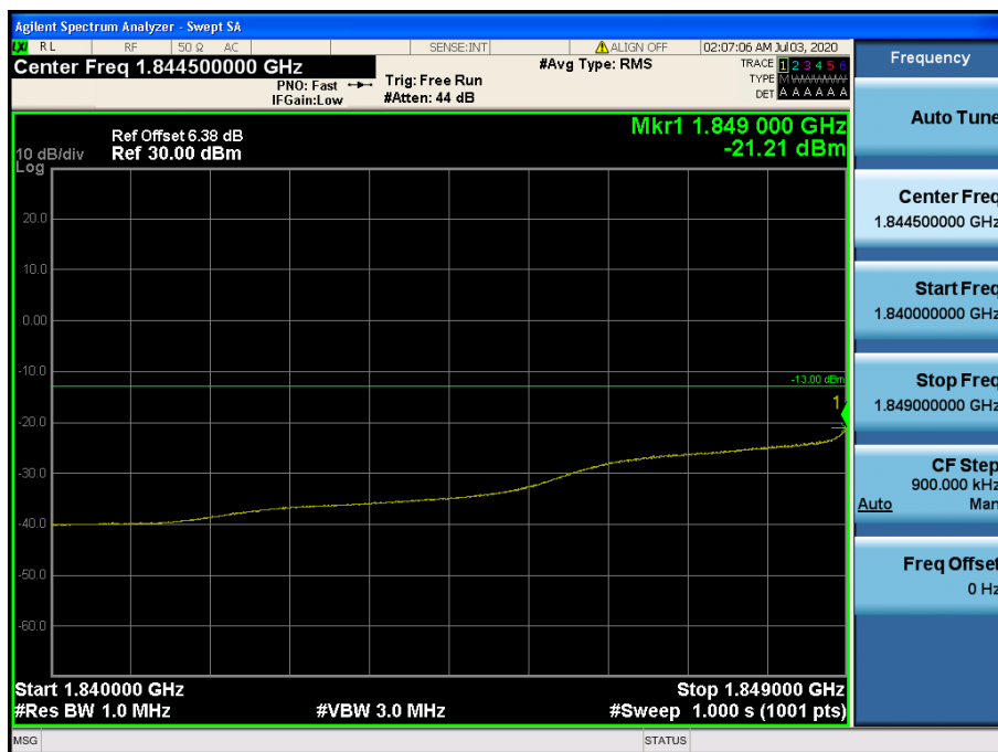
LTE Band 2 / 10MHz / QPSK - RB Size/Offset (25/0)
