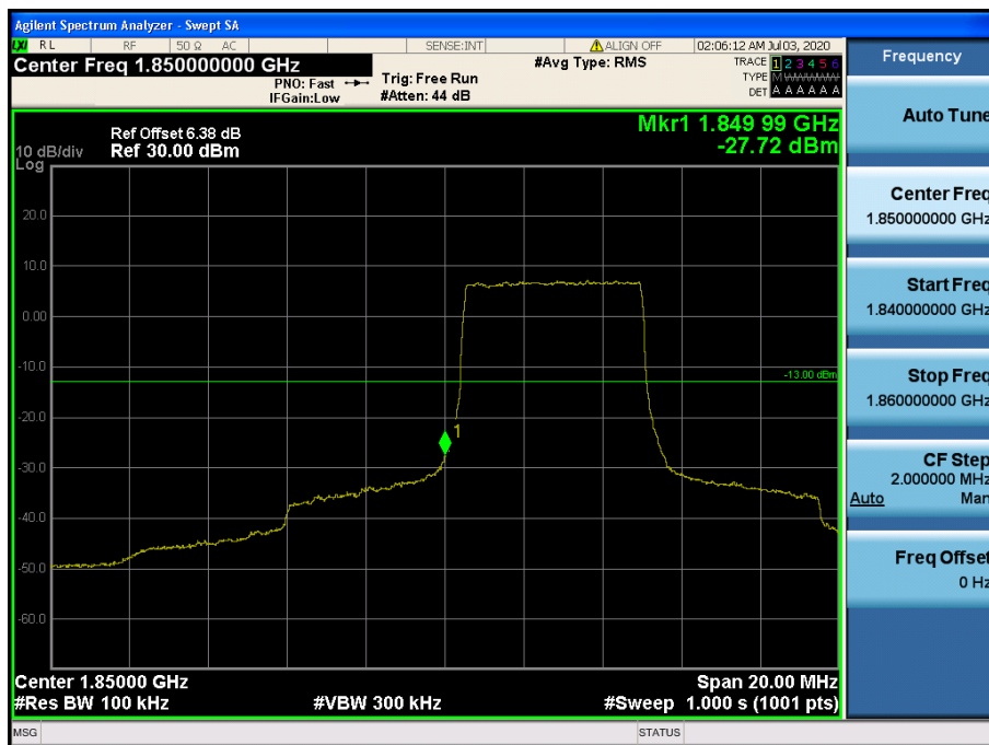
LTE Band 2 / 10MHz / QPSK - RB Size/Offset (25/0)
