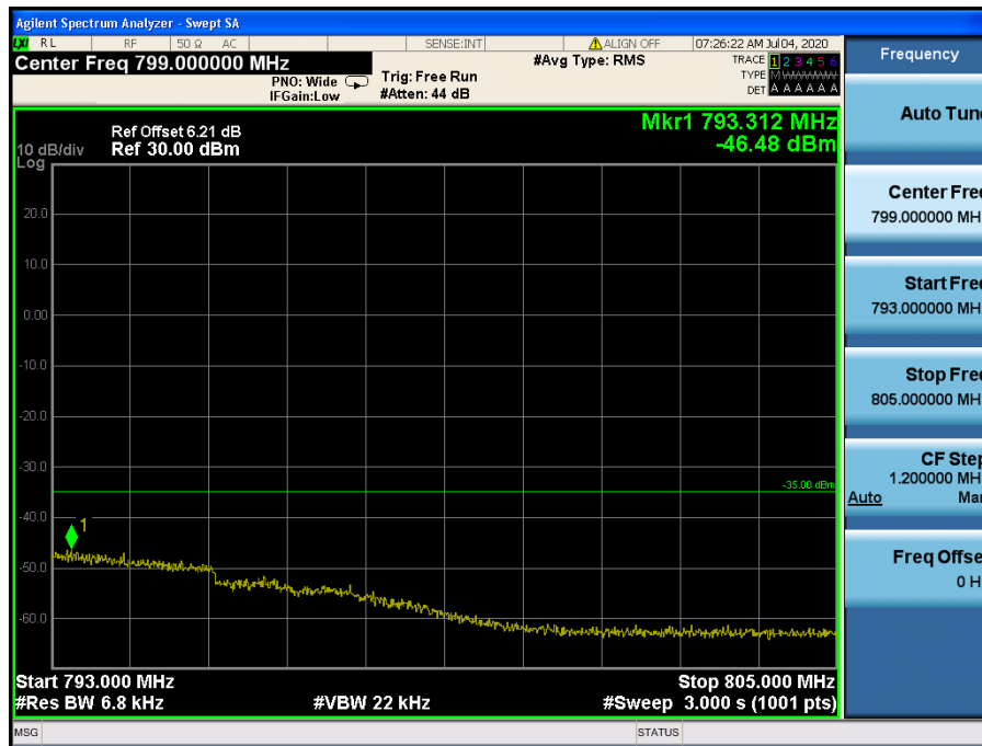
LTE Band 13 / 10MHz / QPSK - RB Size/Offset (50/0)
