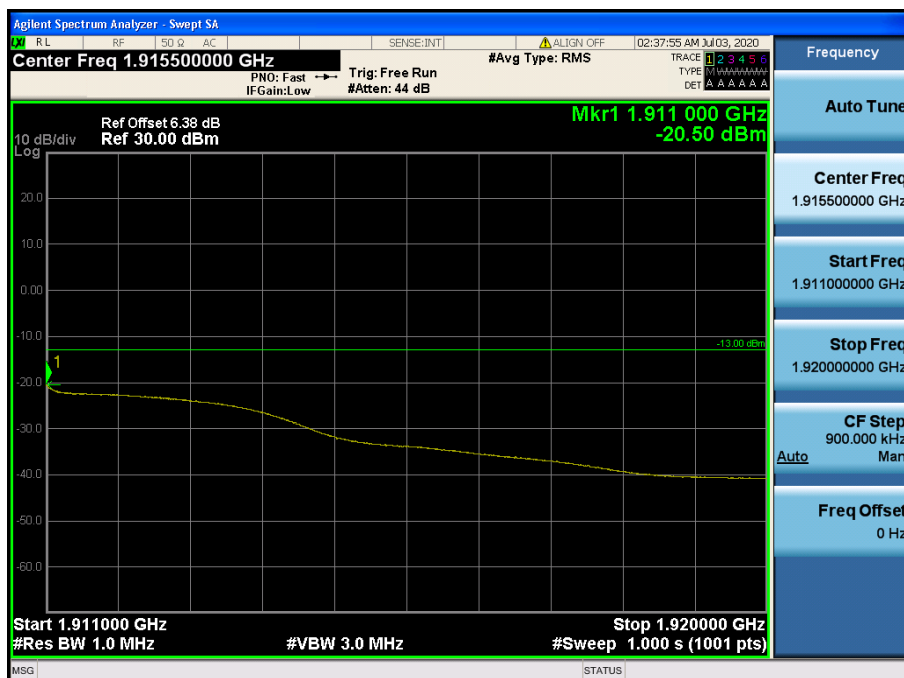
LTE Band 2 / 10MHz / QPSK - RB Size/Offset (25/25)
