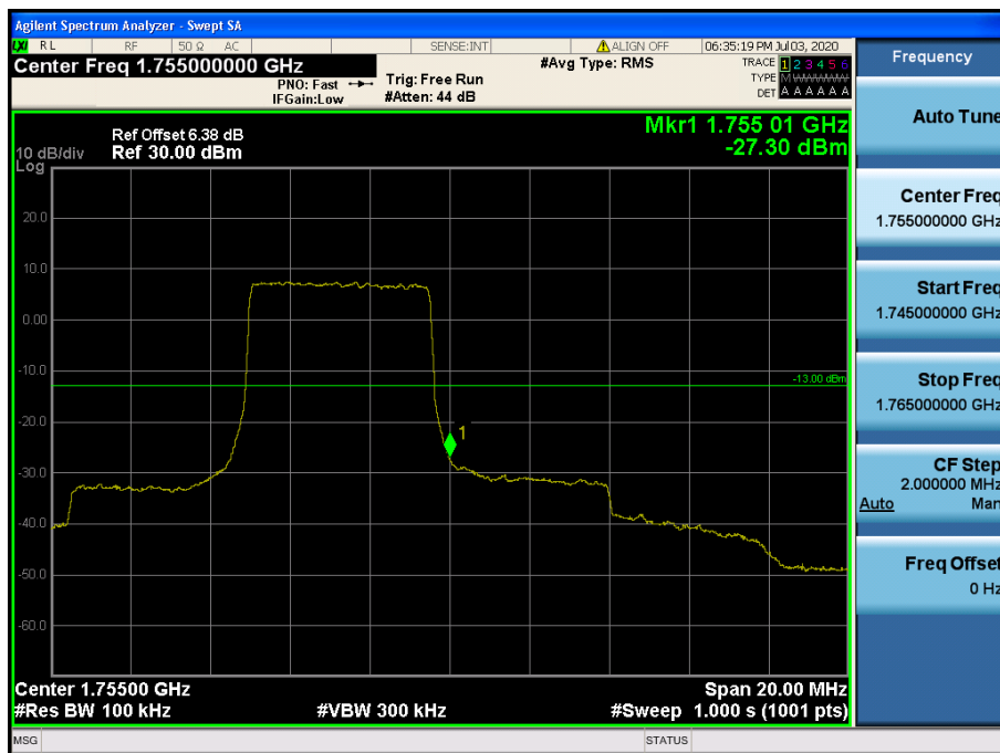
LTE Band 4 / 10MHz / QPSK - RB Size/Offset (25/25)
