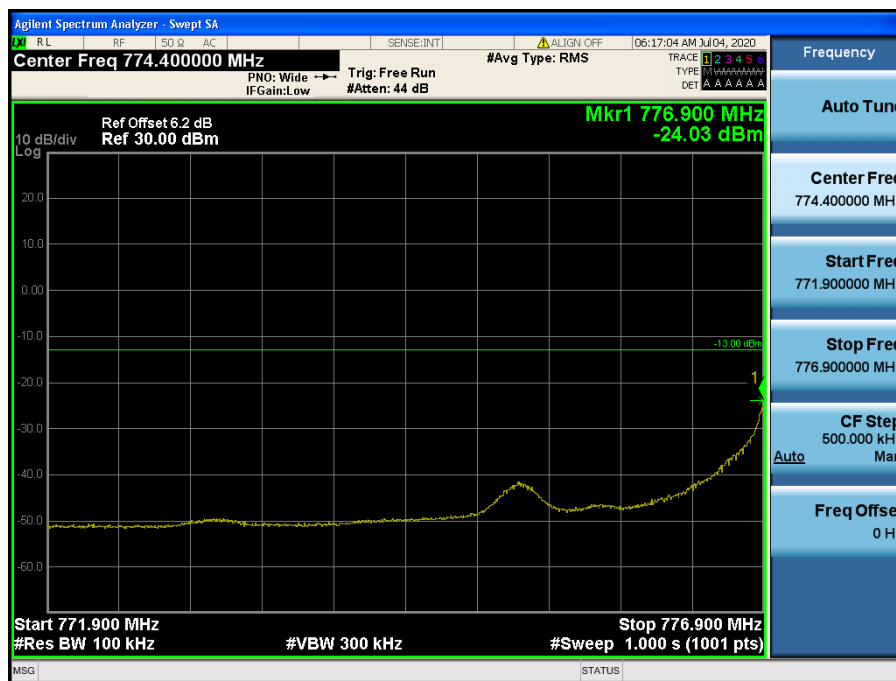
LTE Band 13 / 5MHz / QPSK - RB Size/Offset (1/0)
