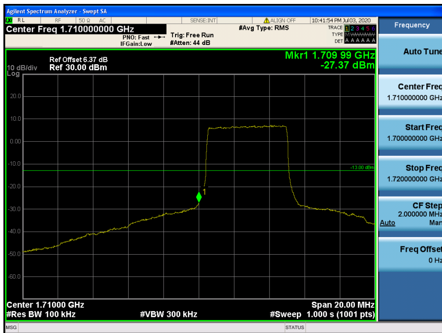
LTE Band 4 / 10MHz / 16QAM - RB Size/Offset (25/0)
