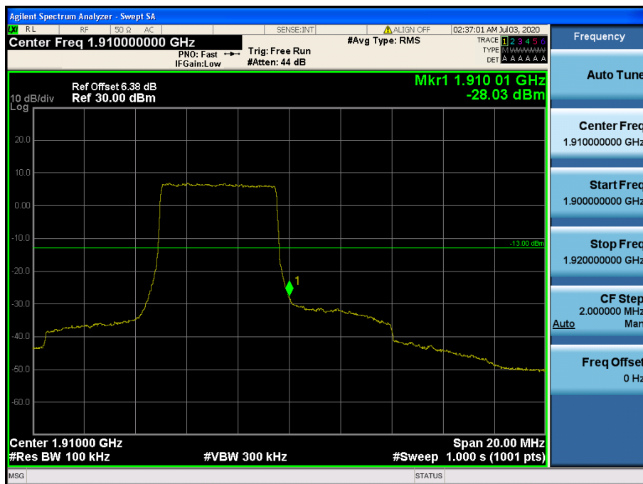
LTE Band 2 / 10MHz / QPSK - RB Size/Offset (25/25)
