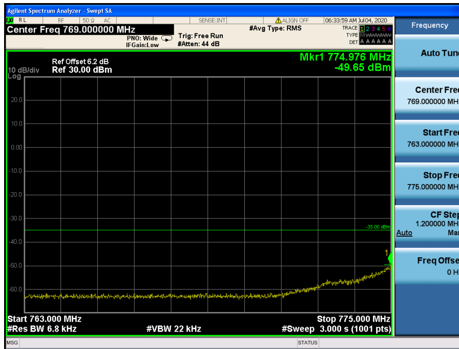
LTE Band 13 / 5MHz / QPSK - RB Size/Offset (25/0)
