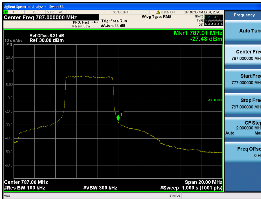
LTE Band 13 / 10MHz / QPSK - RB Size/Offset (25/25)
