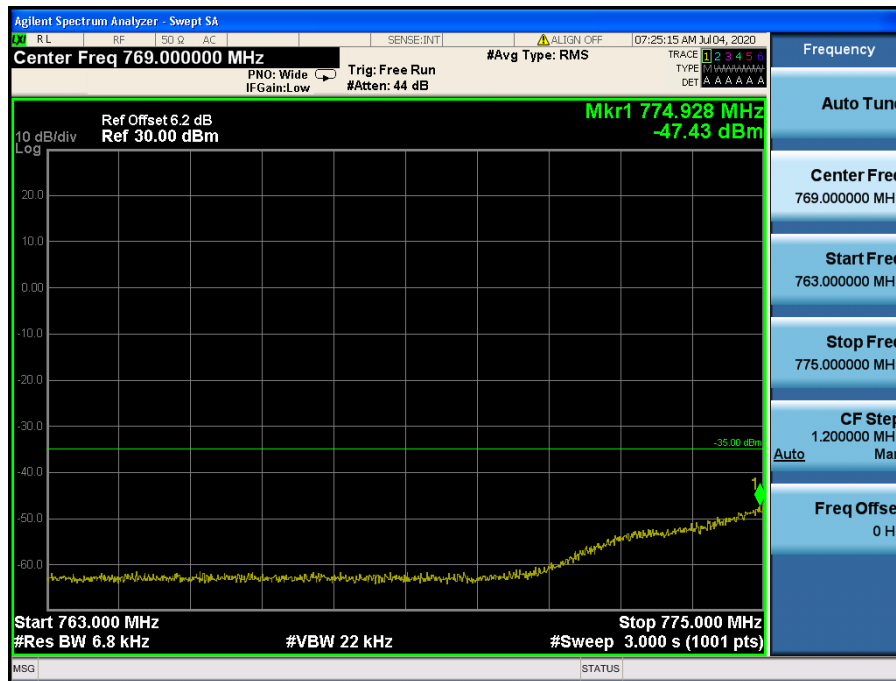
LTE Band 13 / 10MHz / QPSK – RB Size/Offset (25/0)
