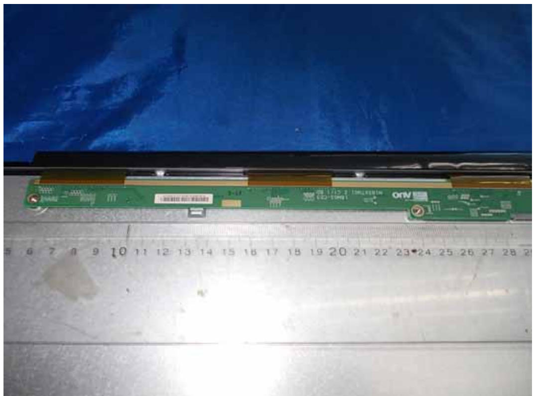
FIGURE 12 LCD MONITOR (M/N: LS1920wG) LCD PANEL BOARD (SOLDERED SIDE #2)
