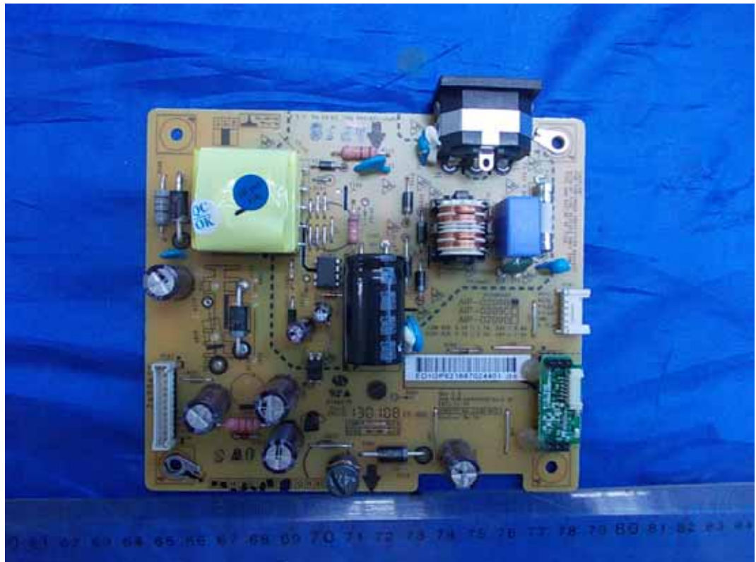
FIGURE 2 LCD MONITOR (M/N: LS1920wG) POWER BOARD (COMPONENT SIDE)
