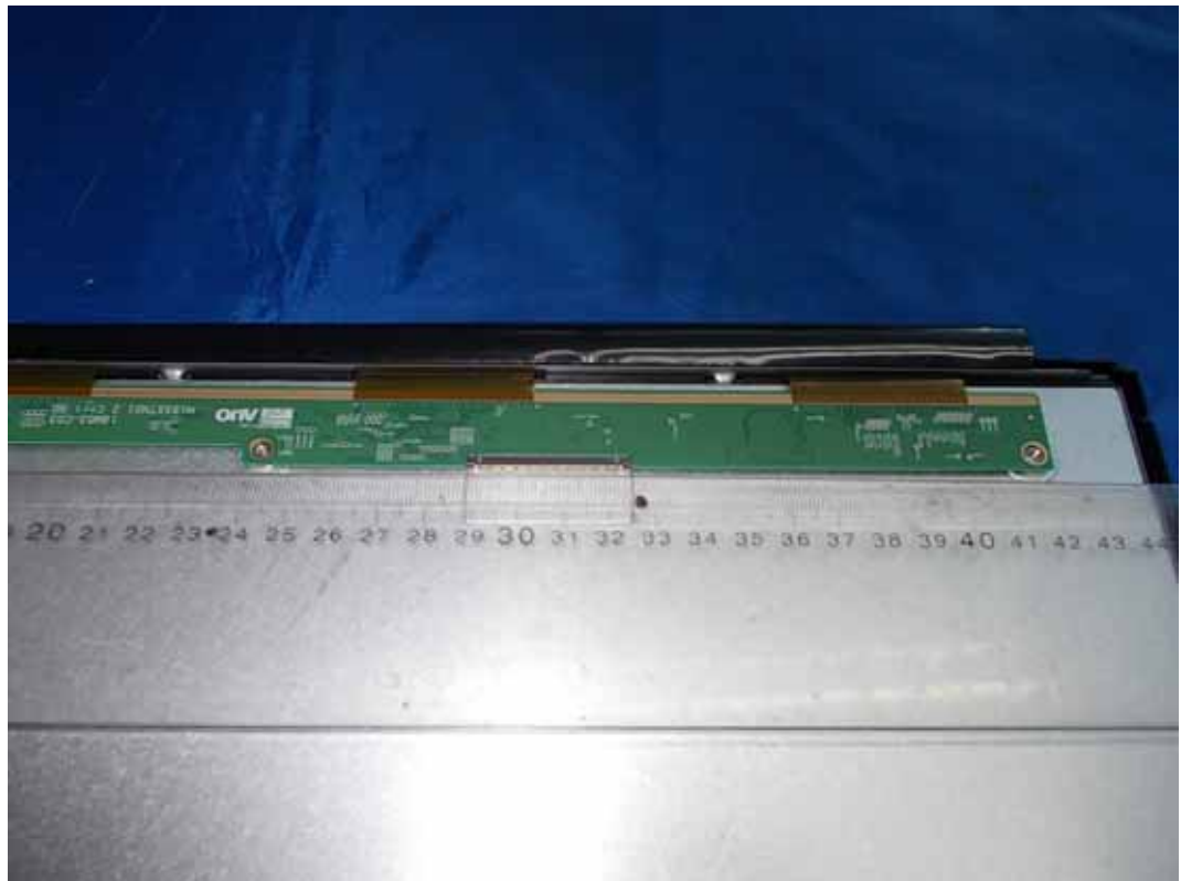
FIGURE 11 LCD MONITOR (M/N: LS1920wG) LCD PANEL BOARD (SOLDERED SIDE #1)
