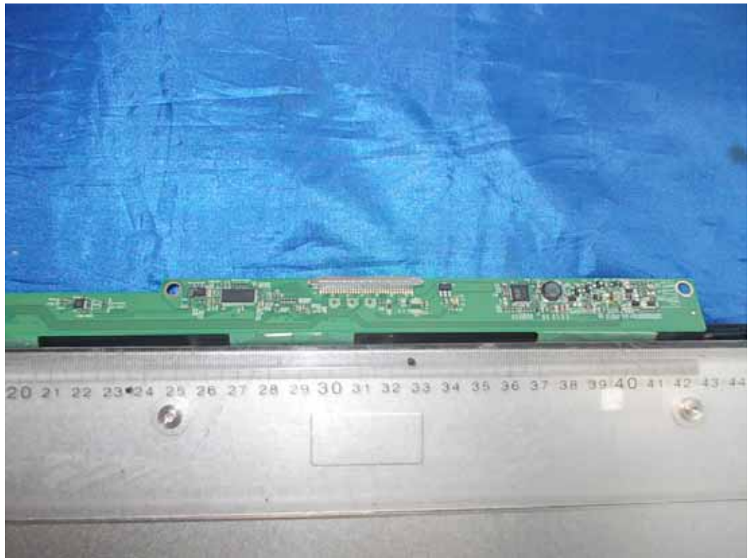
FIGURE 9 LCD MONITOR (M/N: LS1920wG) LCD PANEL BOARD (COMPONENT SIDE #1)
