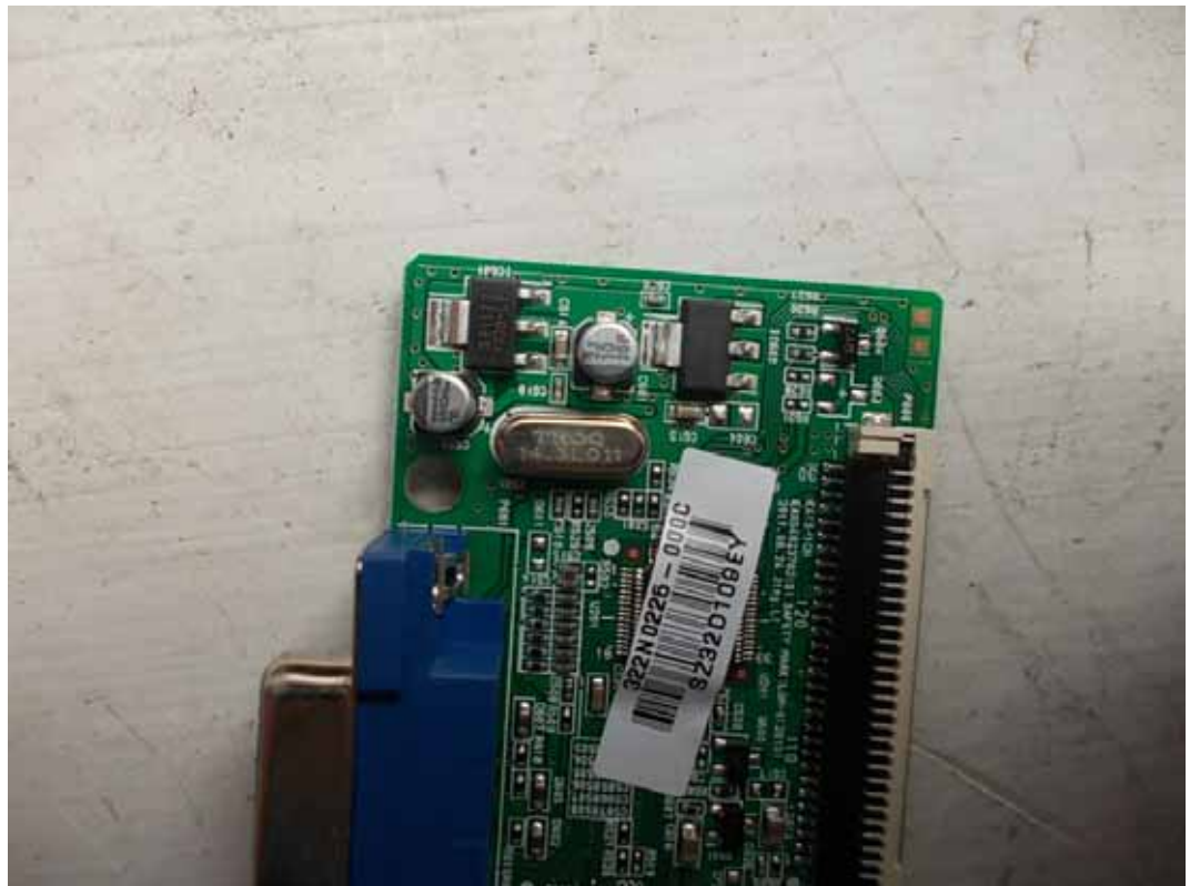
FIGURE 6 LCD MONITOR (M/N: LS1920wG) CRYSTAL ON MAIN BOARD
