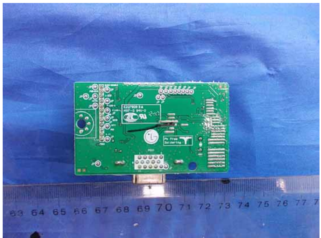
FIGURE 5 LCD MONITOR (M/N: LS1920wG) MAIN BOARD (SOLDERED SIDE)
