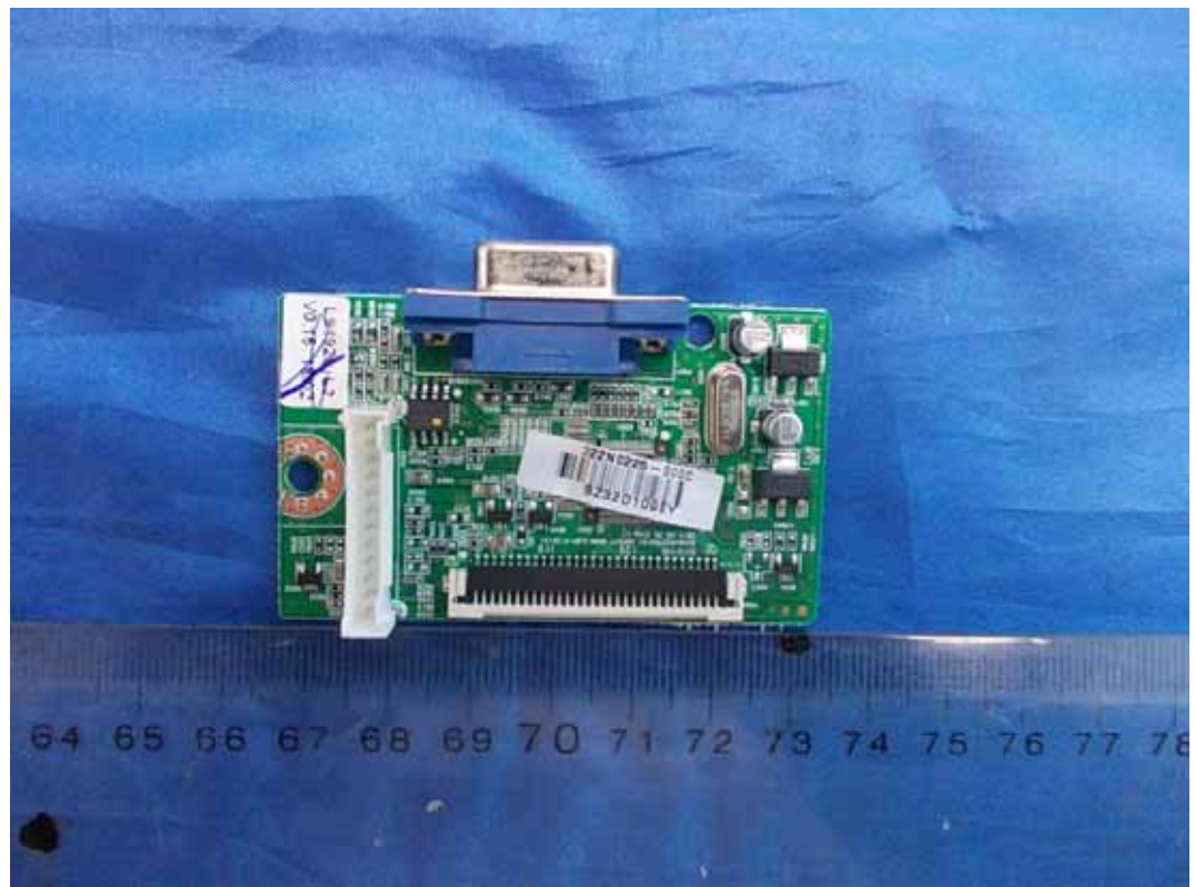
FIGURE 4 LCD MONITOR (M/N: LS1920wG) MAIN BOARD (COMPONENT SIDE)
