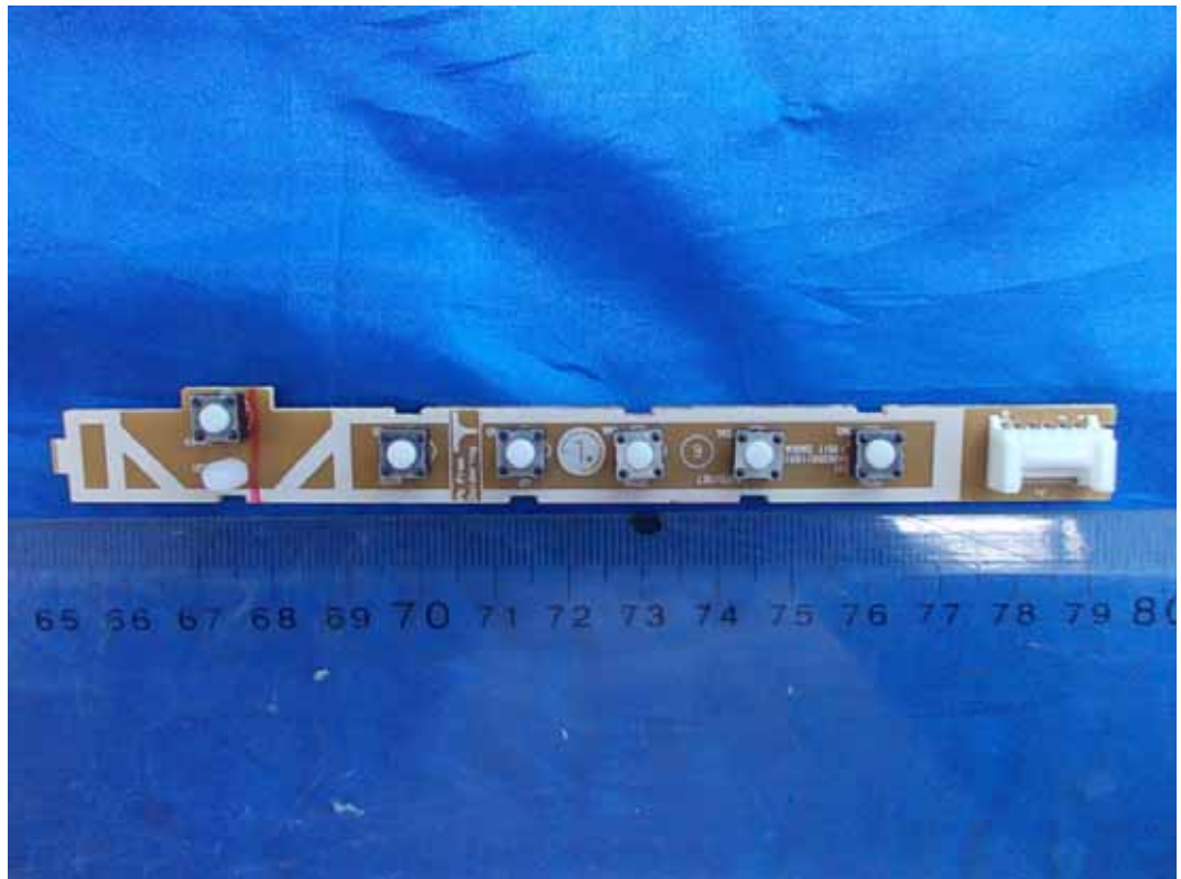
FIGURE 7 LCD MONITOR (M/N: LS1920wG) KEY BOARD (COMPONENT SIDE)
