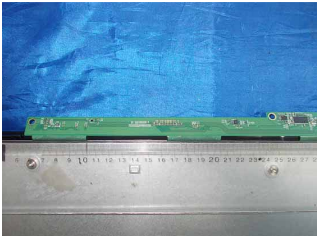
FIGURE 10 LCD MONITOR (M/N: LS1920wG) LCD PANEL BOARD (COMPONENT SIDE #2)
