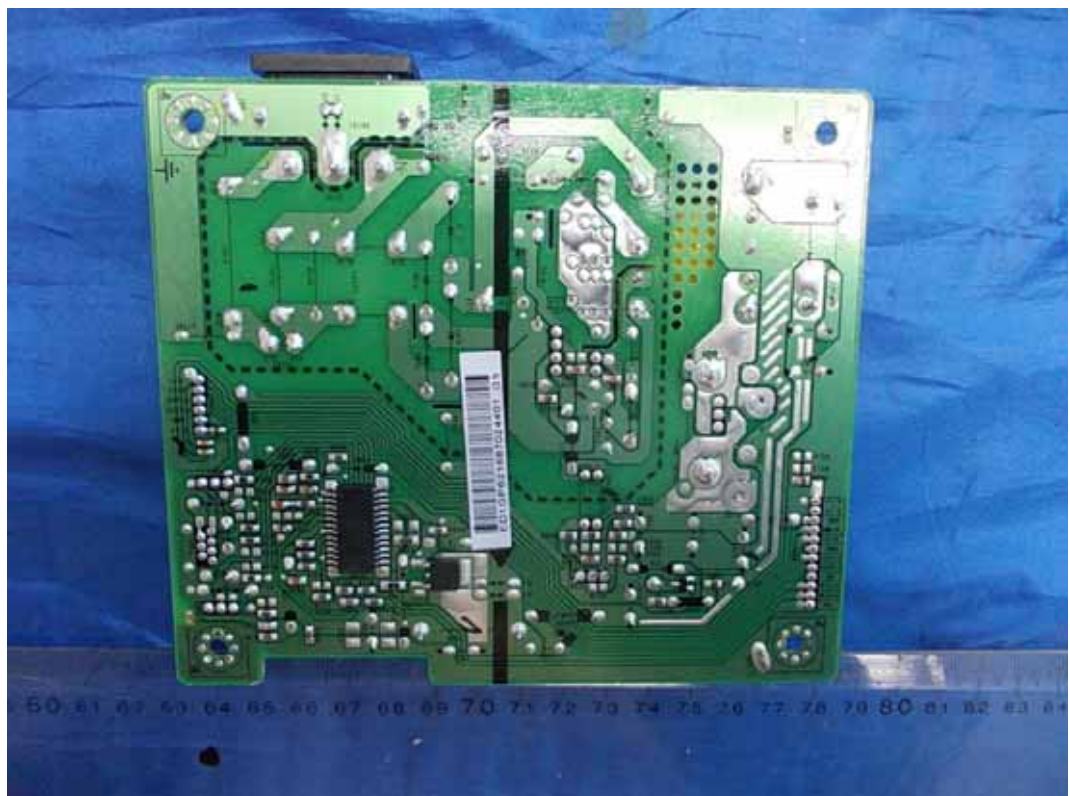
FIGURE 3 LCD MONITOR (M/N: LS1920wG) POWER BOARD (SOLDERED SIDE)
