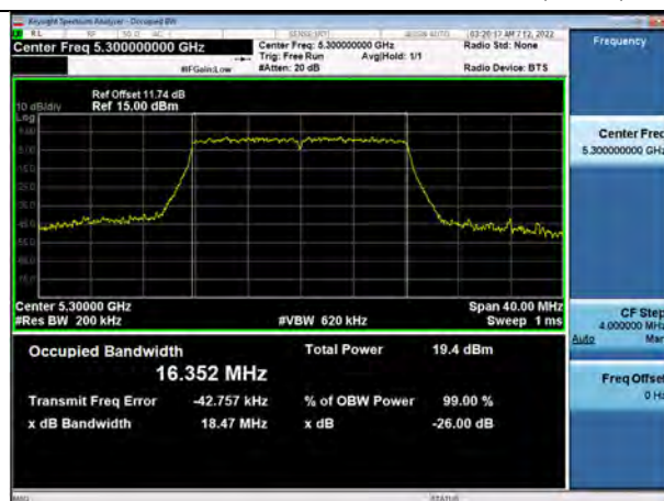
802.11a UNII 3 BAND 26dB Bandwidth (CH 165)
