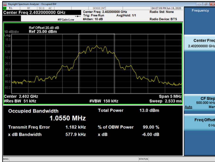
99 % Bandwidth plot (Low-CH 0)
