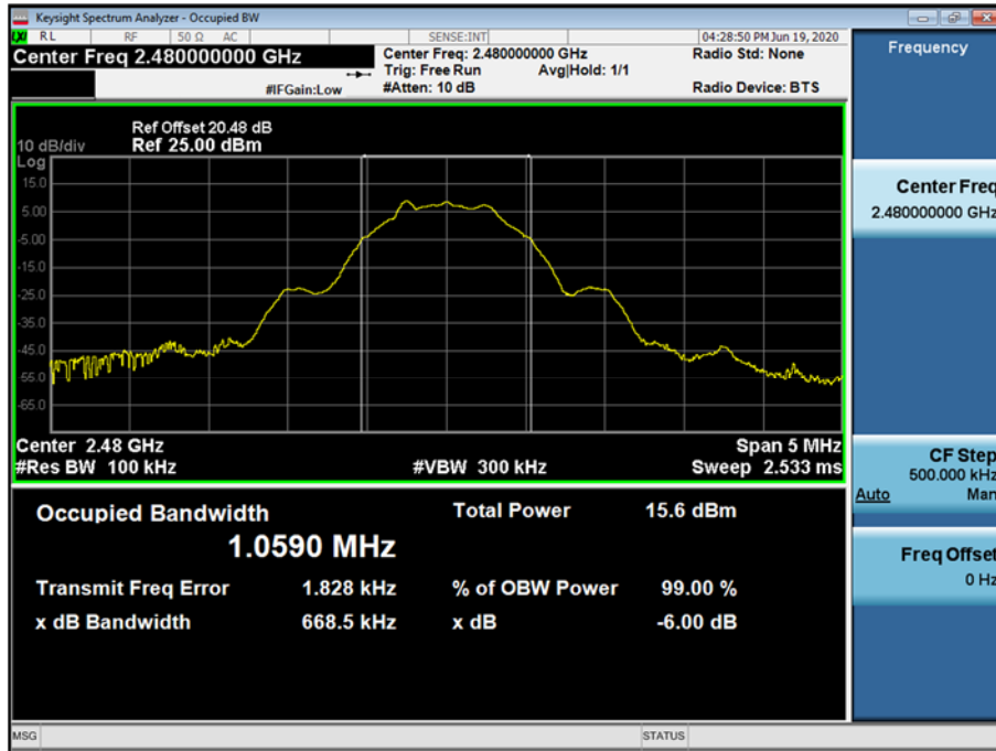
6 dB Bandwidth plot (High-CH 39)
