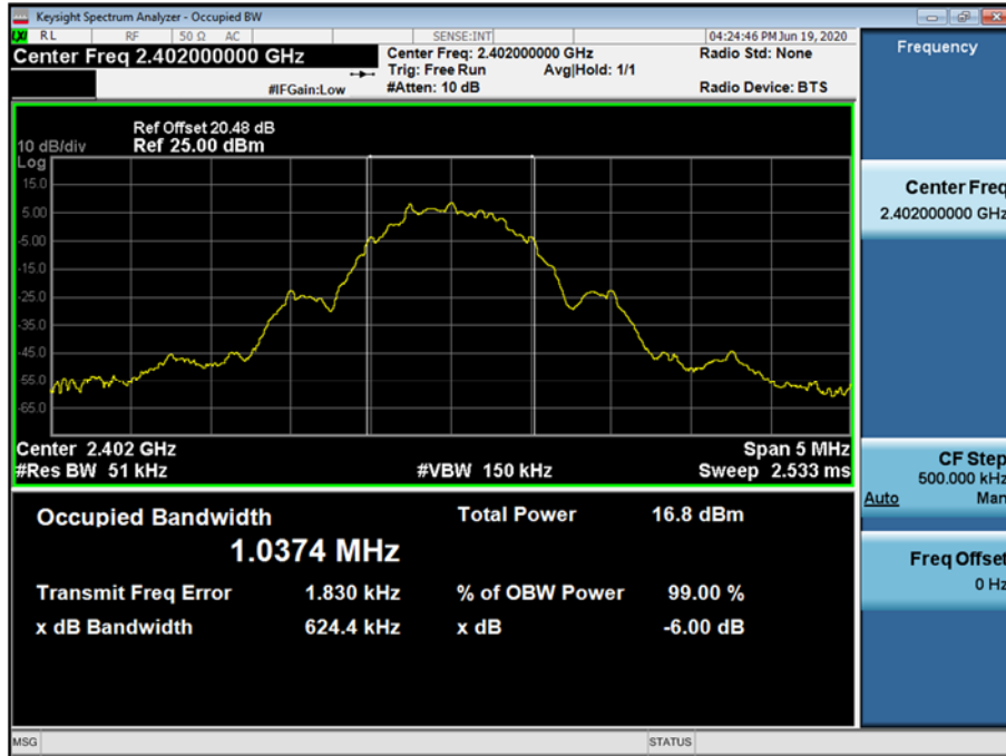
99 % Bandwidth plot (Low-CH 0)
