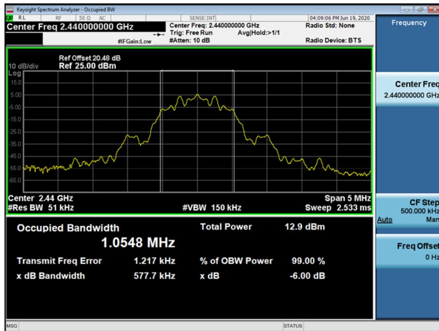
99 % Bandwidth plot (Mid-CH 19)
