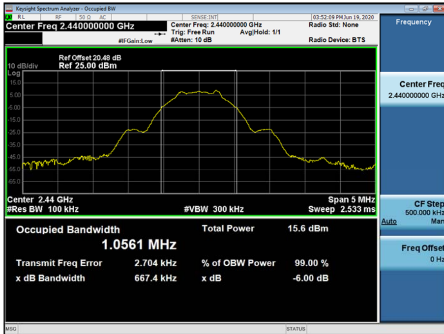
6 dB Bandwidth plot (Mid-CH 19)
