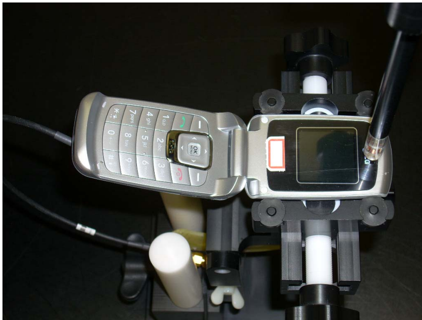
Figure 12-1 Test Setup for Wireless Device
