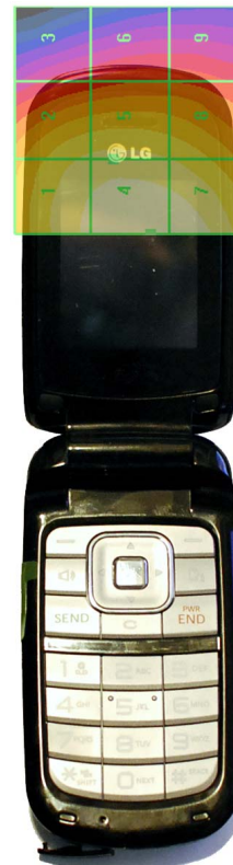
Figure 17-5 H-Field WD Scan overlay
