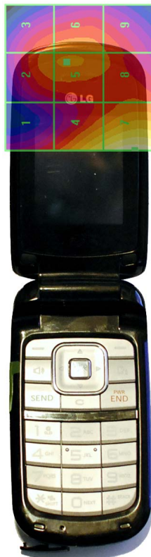
Figure 17-4 E-Field WD Scan overlay
