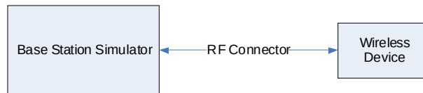
Figure 14-1 Power Measurement Setup
