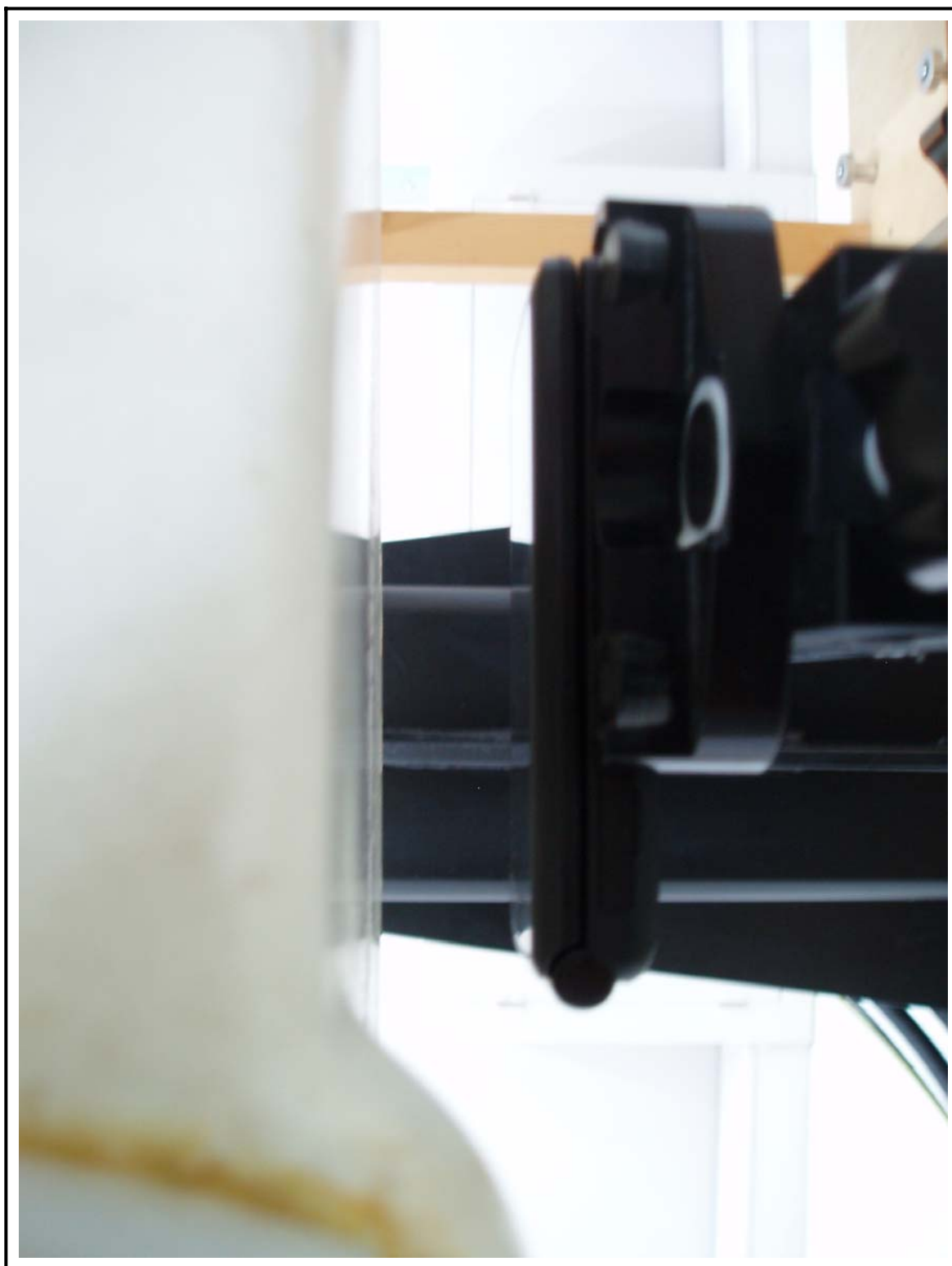
Figure 5 Body SAR Test Setup – w/o Holster
