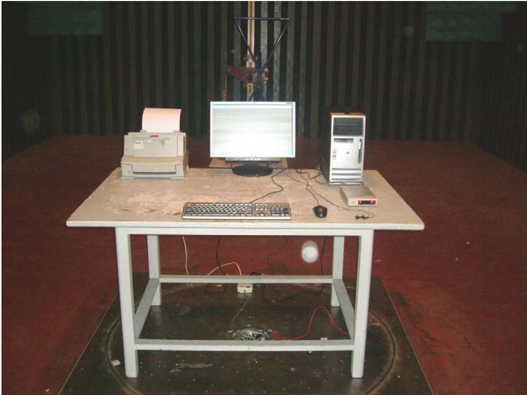
FRONT VIEW OF RADIATED EMISSION TEST (LOW FREQUENCY)
