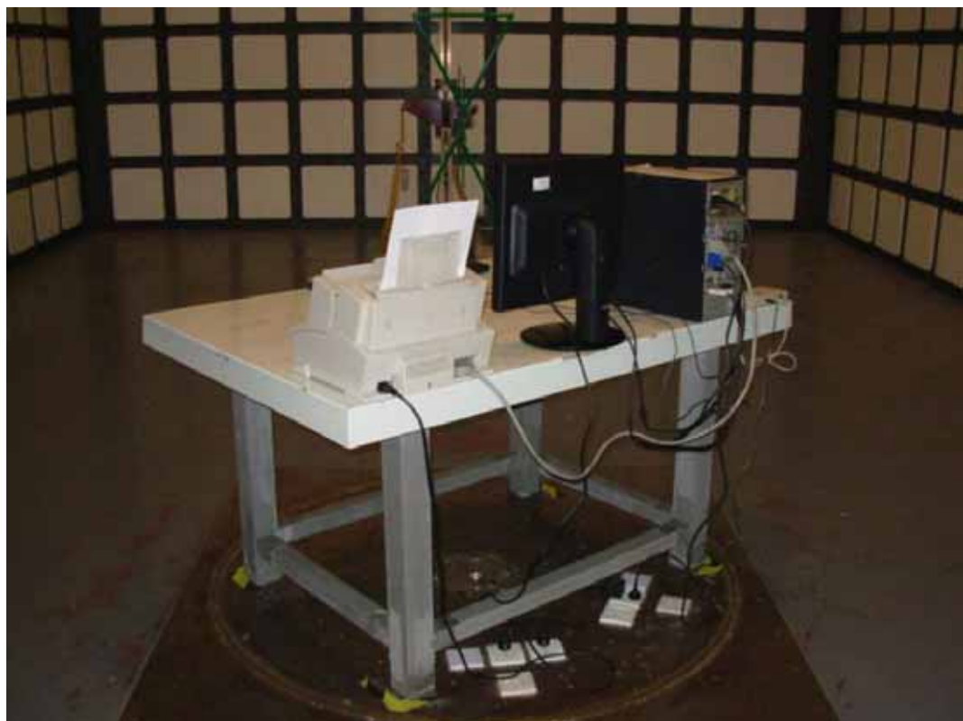
SETUP WITH MAXIMUM DETECTED EMISSION AT VERTICAL POLARIZATION (DVI 1024*768@60Hz (Rotate 90 degree))
