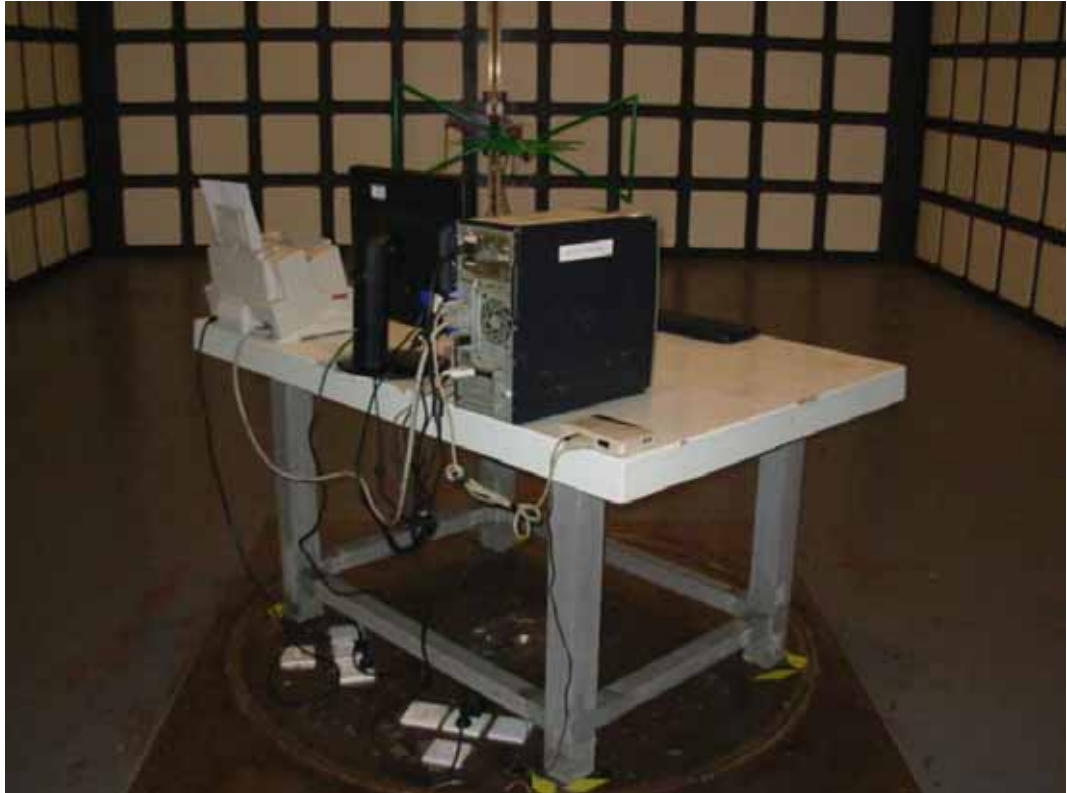
SETUP WITH MAXIMUM DETECTED EMISSION AT HORIZONTAL POLARIZATION (DVI 1020*768@60Hz (Rotate 90 degree))
