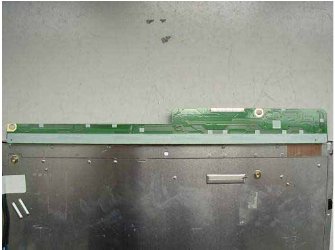
FIGURE 15 LCD MONITOR (M/N: L1942PQT) LCD PANEL MAIN BOARD (SOLDERED SIDE)
