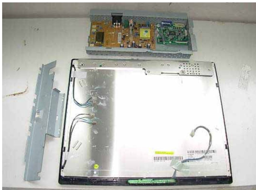
FIGURE 2 LCD MONITOR (M/N: L1942PQT) BOARDS REMOVED
