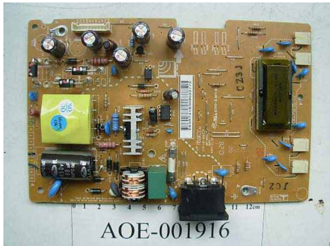
FIGURE 9 LCD MONITOR (M/N: L1942PQT) POWER BOARD (COMPONENT SIDE)
