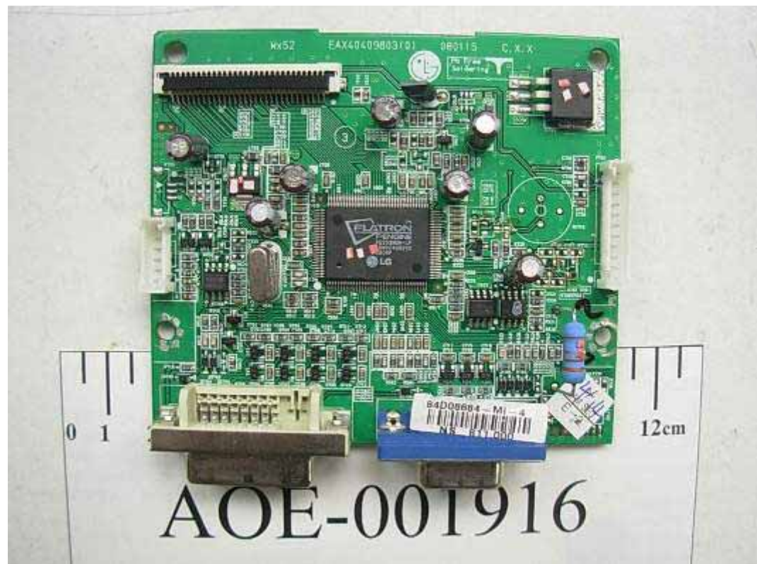
FIGURE 5 LCD MONITOR (M/N: L1942PQT) MAIN BOARD (COMPONENT SIDE)
