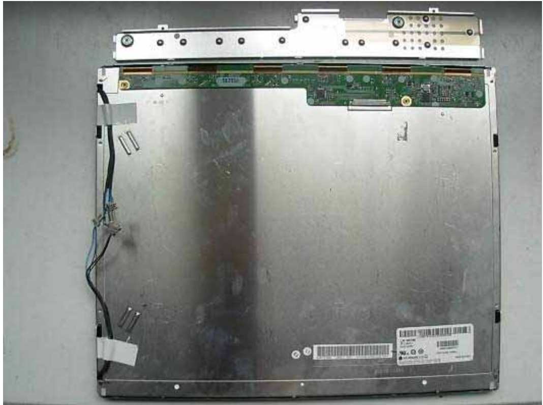
FIGURE 13 LCD MONITOR (M/N: L1942PQT) LCD PANEL MAIN BOARD COVER REMOVED
