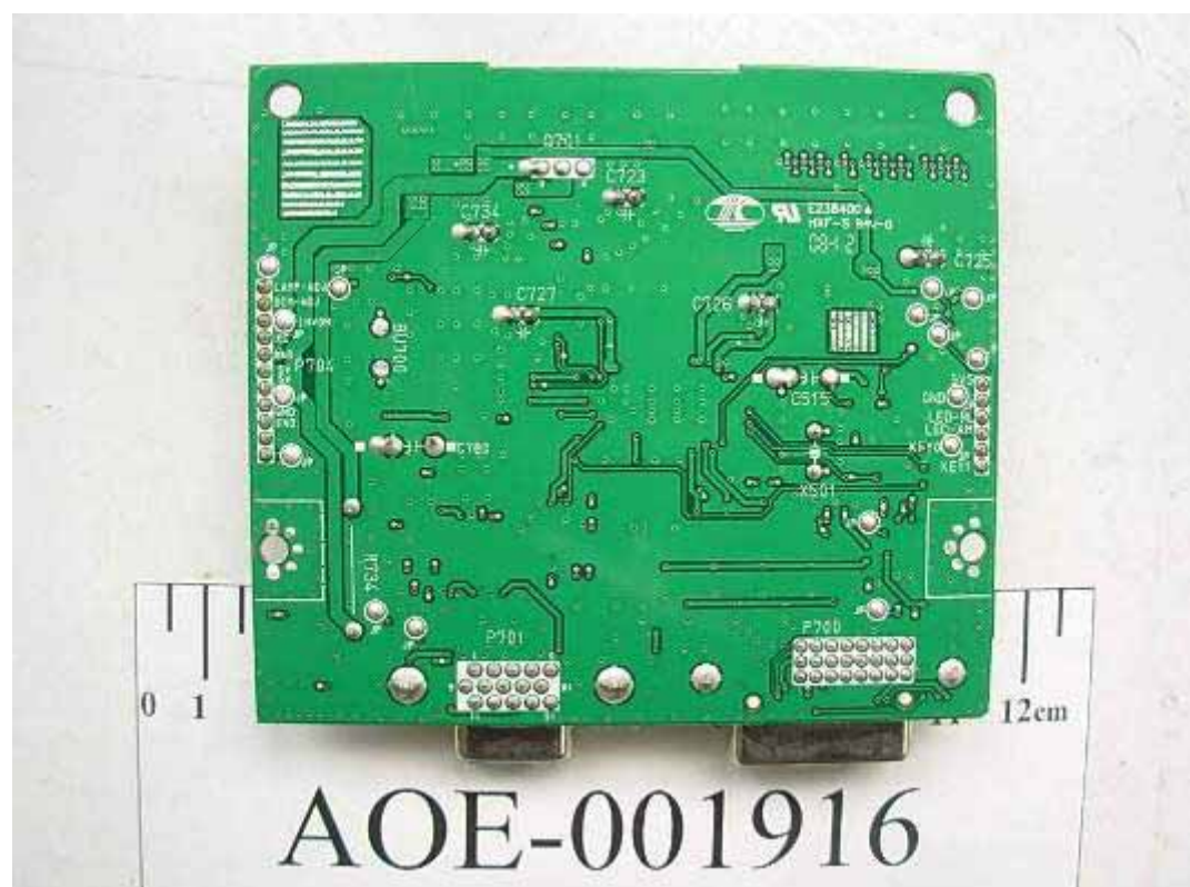
FIGURE 6 LCD MONITOR (M/N: L1942PQT) MAIN BOARD (SOLDERED SIDE)
