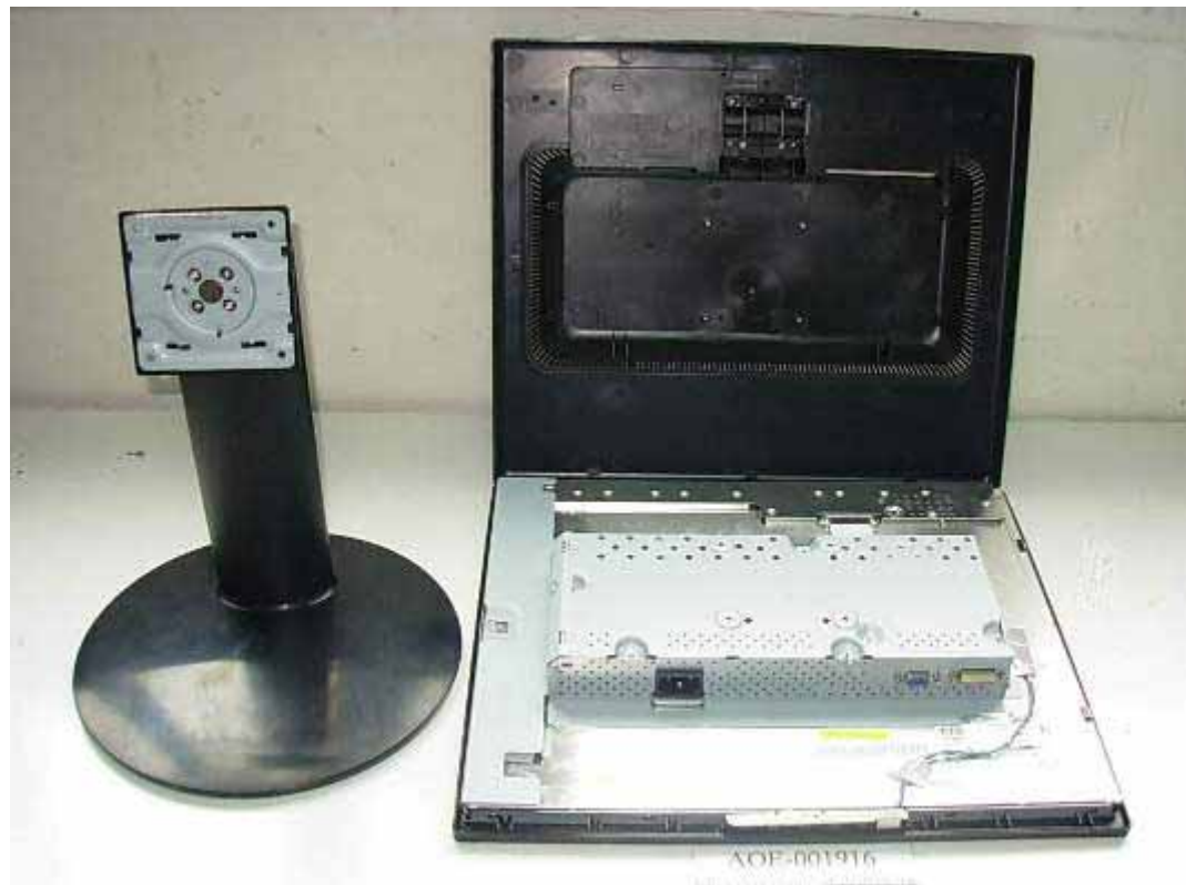
FIGURE 1 LCD MONITOR (M/N: L1942PQT) COVER REMOVED
