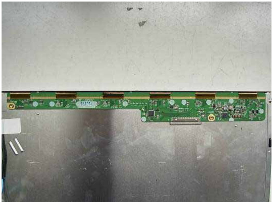
FIGURE 14 LCD MONITOR (M/N: L1942PQT) LCD PANEL MAIN BOARD (COMPONENT SIDE)
