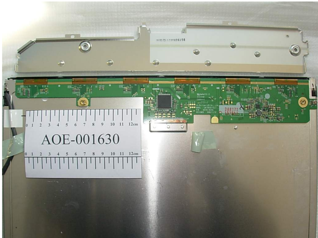
FIGURE 15 LCD MONITOR (M/N: L1755TT) LCD PANEL MAIN BOARD SHIELDED COVER REMOVED
