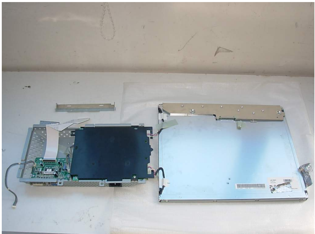
FIGURE 2 LCD MONITOR (M/N: L1755TT) BOARDS REMOVED
