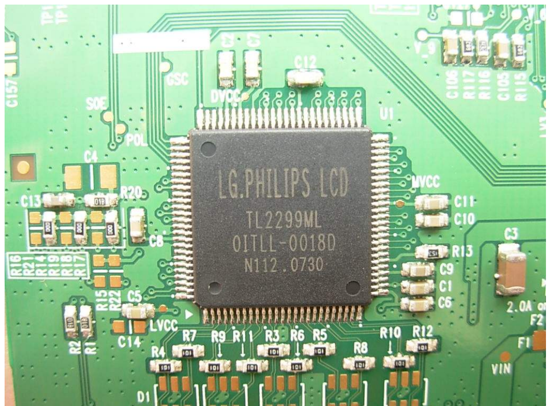
FIGURE 18 LCD MONITOR (M/N: L1755TT) CHIP ON LCD PANEL MAIN BOARD
