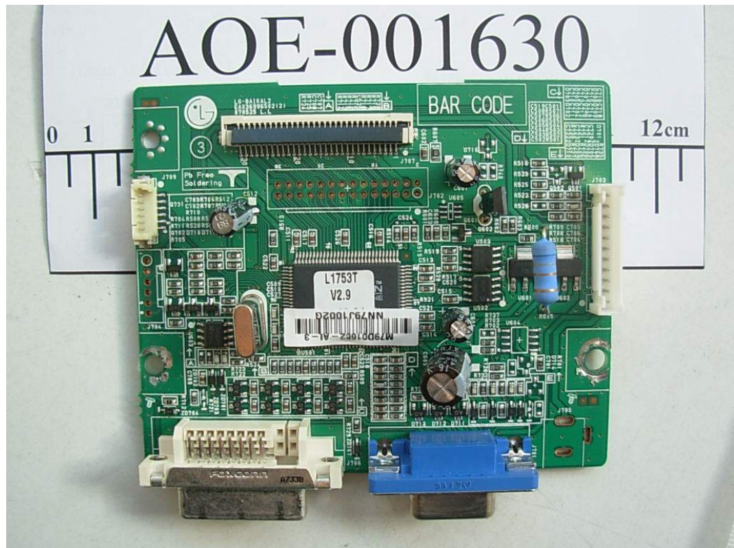
FIGURE 9 LCD MONITOR (M/N: L1755TT) MAIN BOARD (COMPONENT SIDE)
