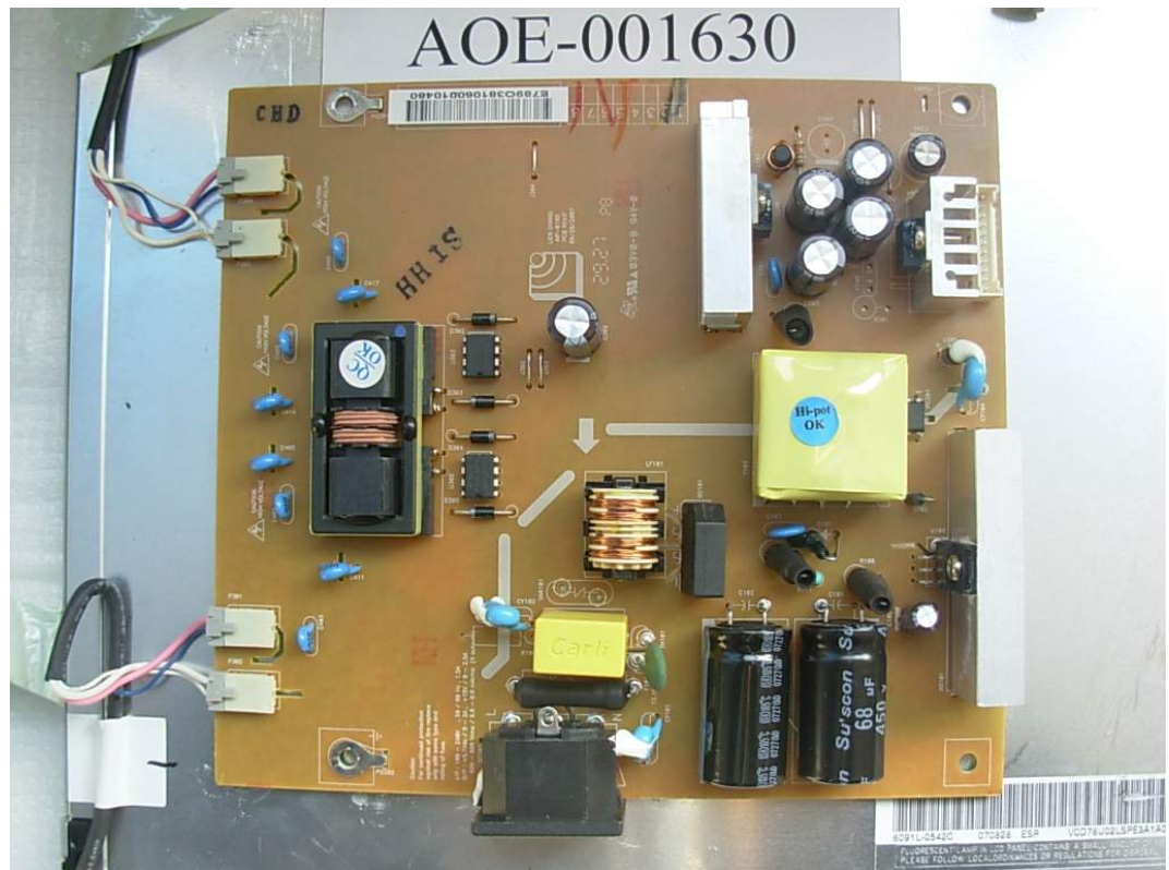
FIGURE 7 LCD MONITOR (M/N: L1755TT) POWER BOARD (COMPONENT SIDE)
