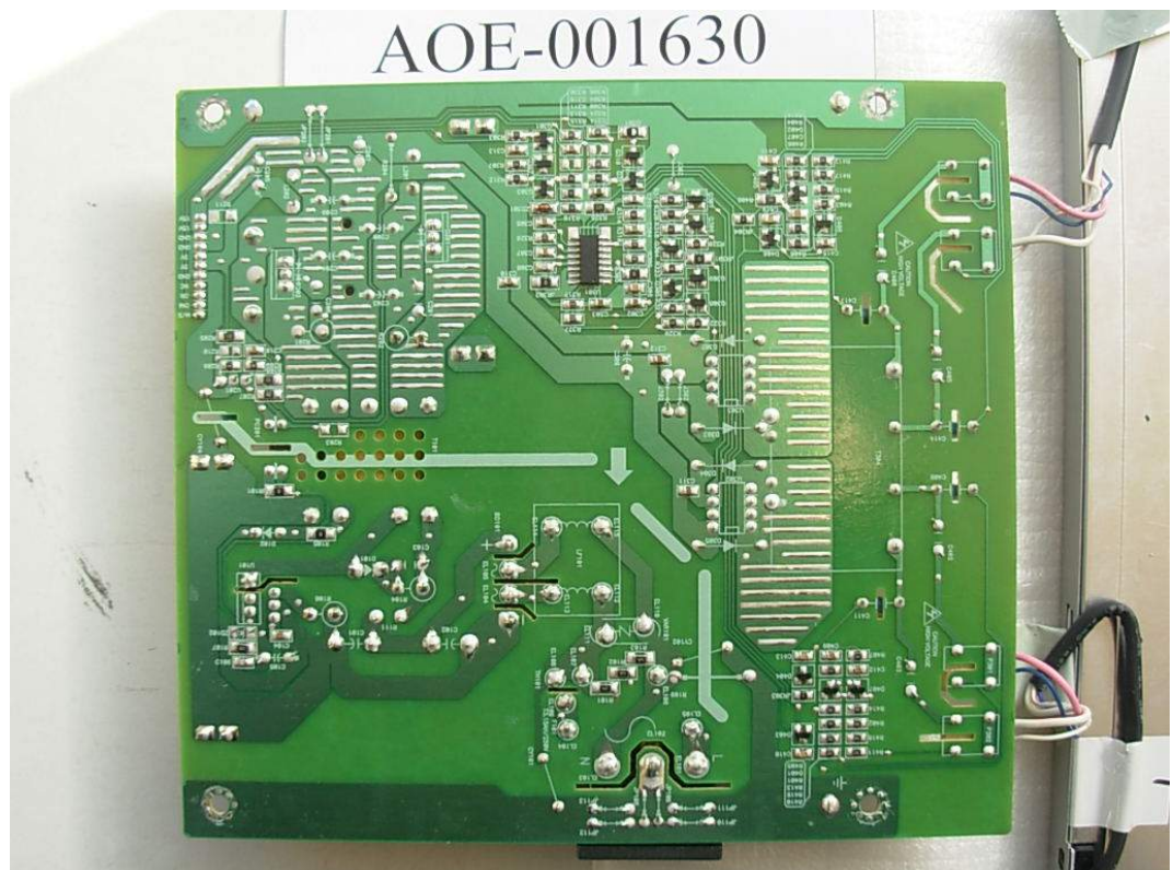
FIGURE 8 LCD MONITOR (M/N: L1755TT) POWER BOARD (SOLDERED SIDE)
