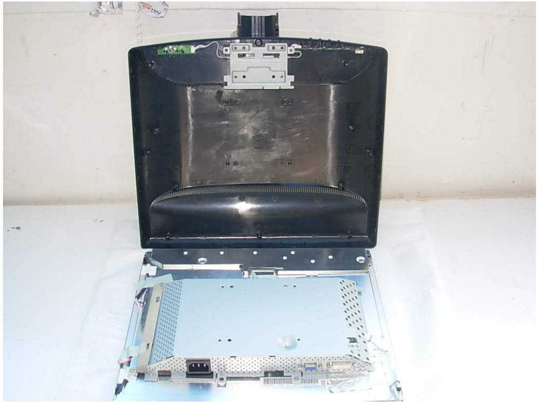
FIGURE 1 LCD MONITOR (M/N: L1755TT) COVER REMOVED
