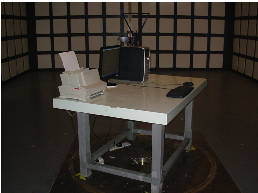
SETUP WITH MAXIMUM DETECTED EMISSION AT VERTICAL POLARIZATION (DVI 1280*1024@60Hz, BELOW 1GHz)
