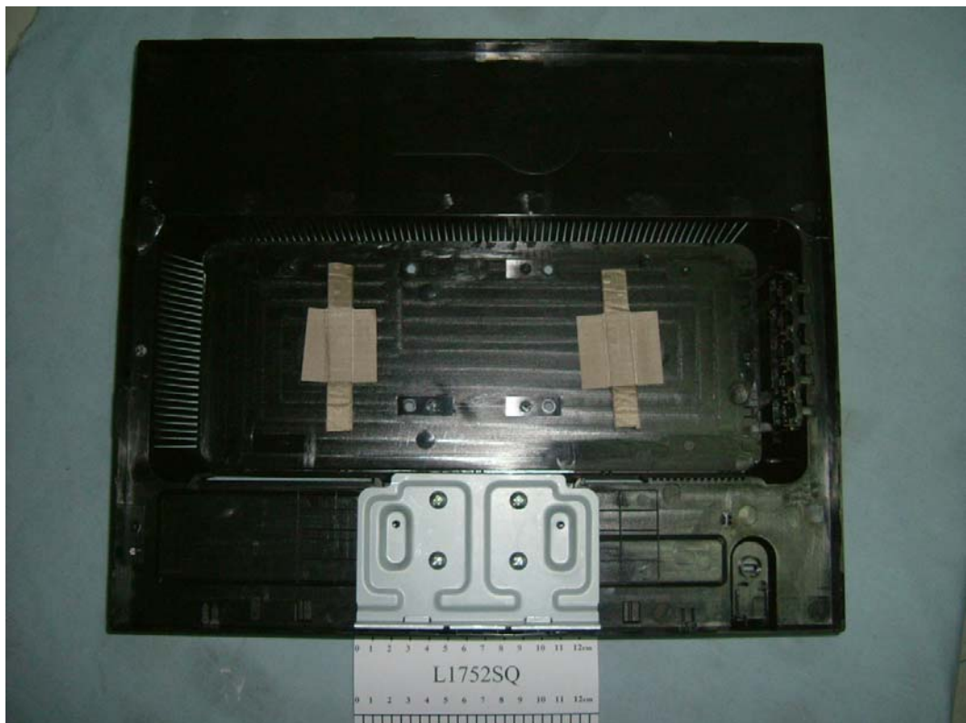
FIGURE 6 LCD MONITOR (M/N: L1752SQ) GASKET IN BACK SHELL
