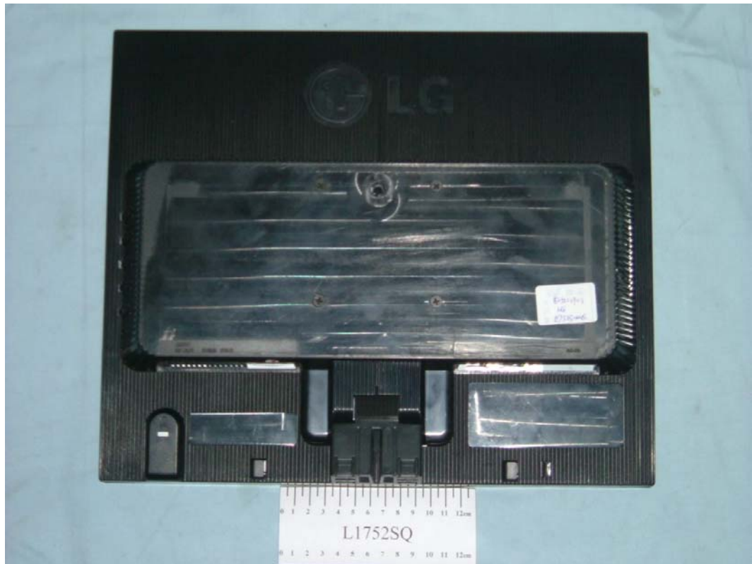
FIGURE 3 LCD MONITOR (M/N: L1752SQ) BOTTOM HOLDER REMOVED
