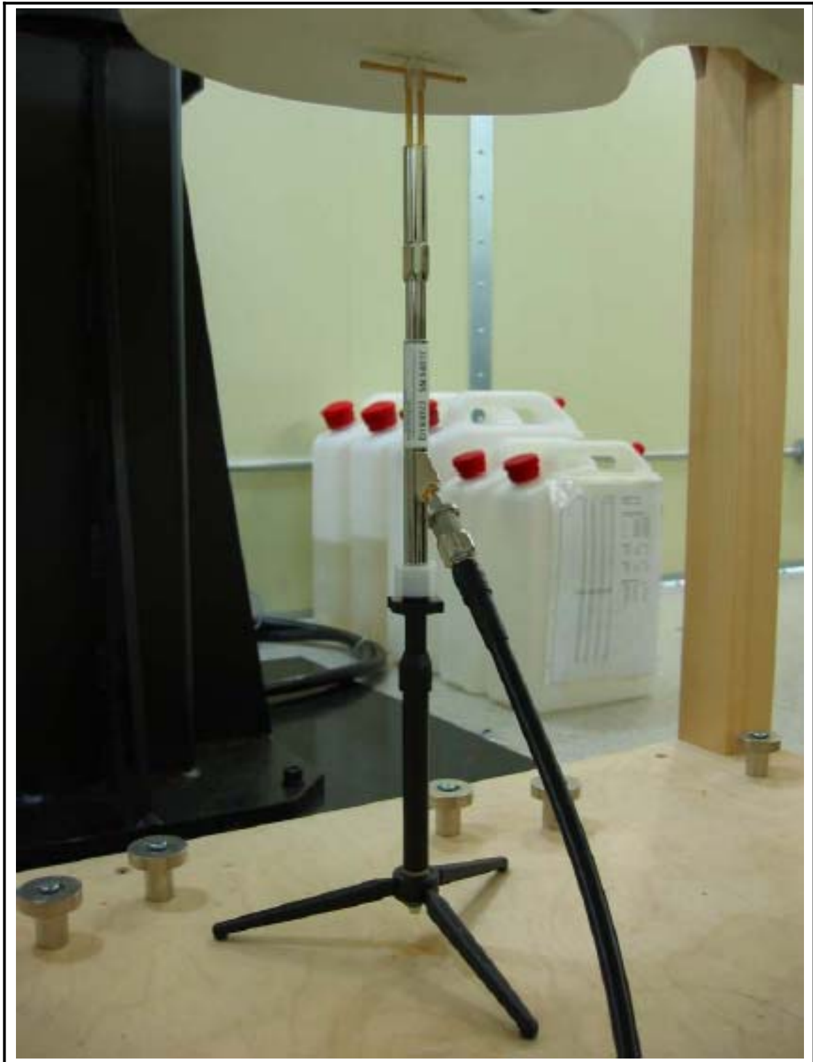
Figure 1 1900 MHz Dipole Validation Test Setup
