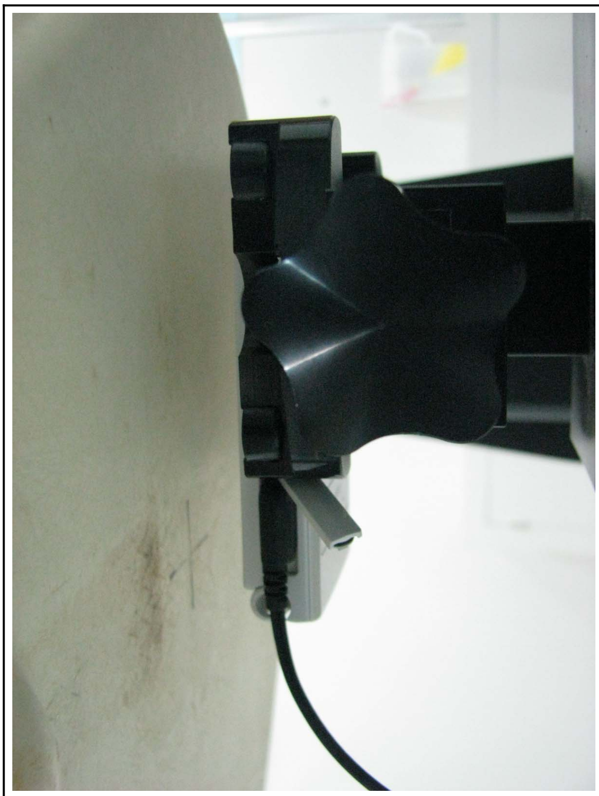
Figure 5 Body SAR Test Setup – w/o Holster
