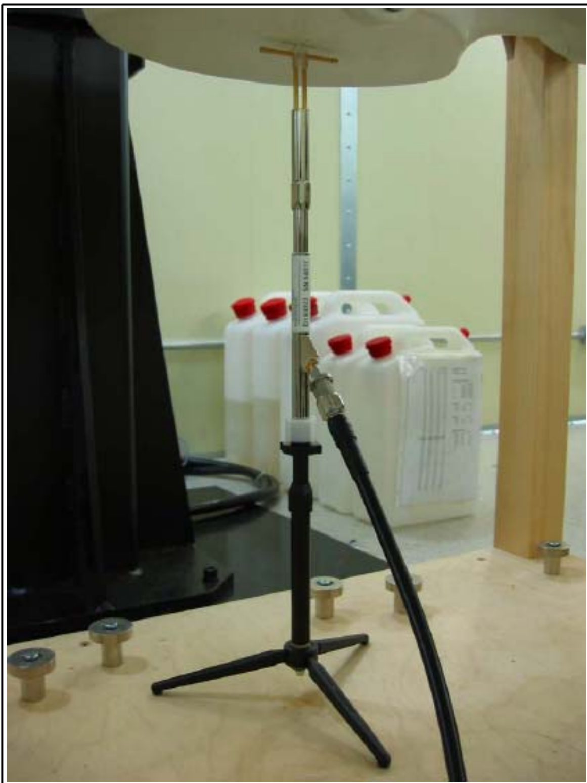
Figure 2 1900 MHz Dipole Validation Test Setup
