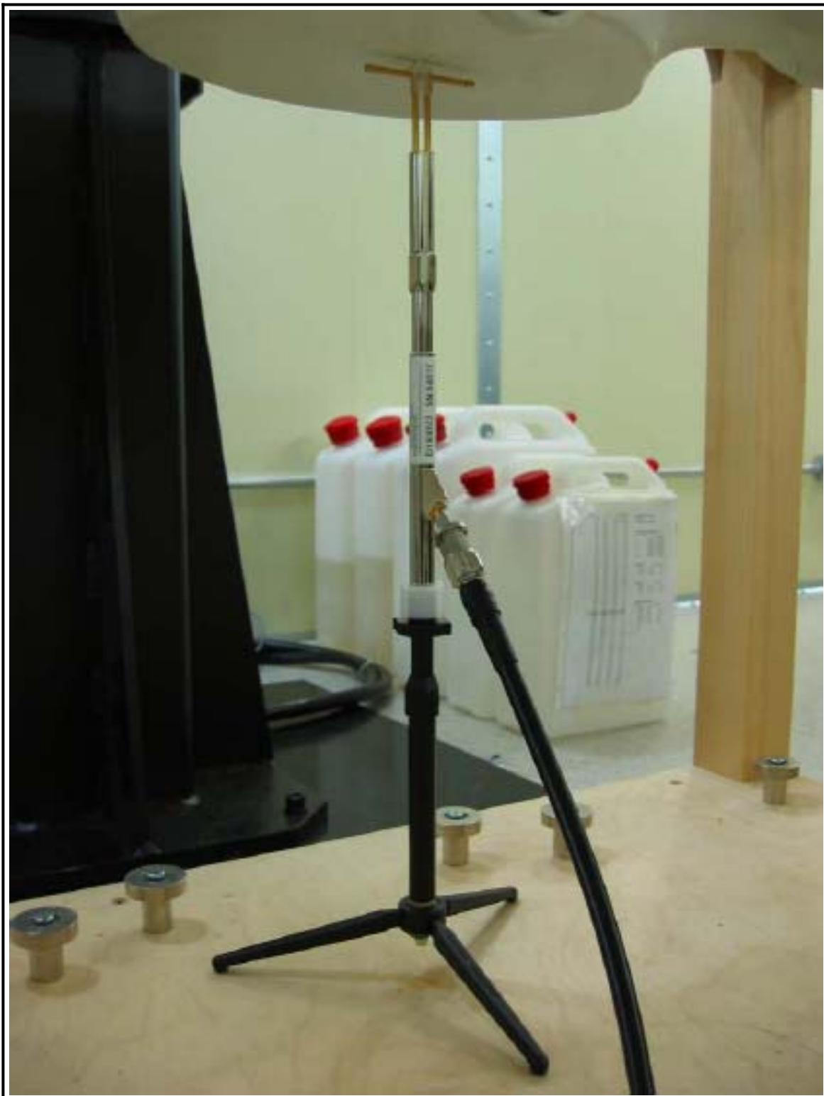
Figure 1 1900 MHz Dipole Validation Test Setup
