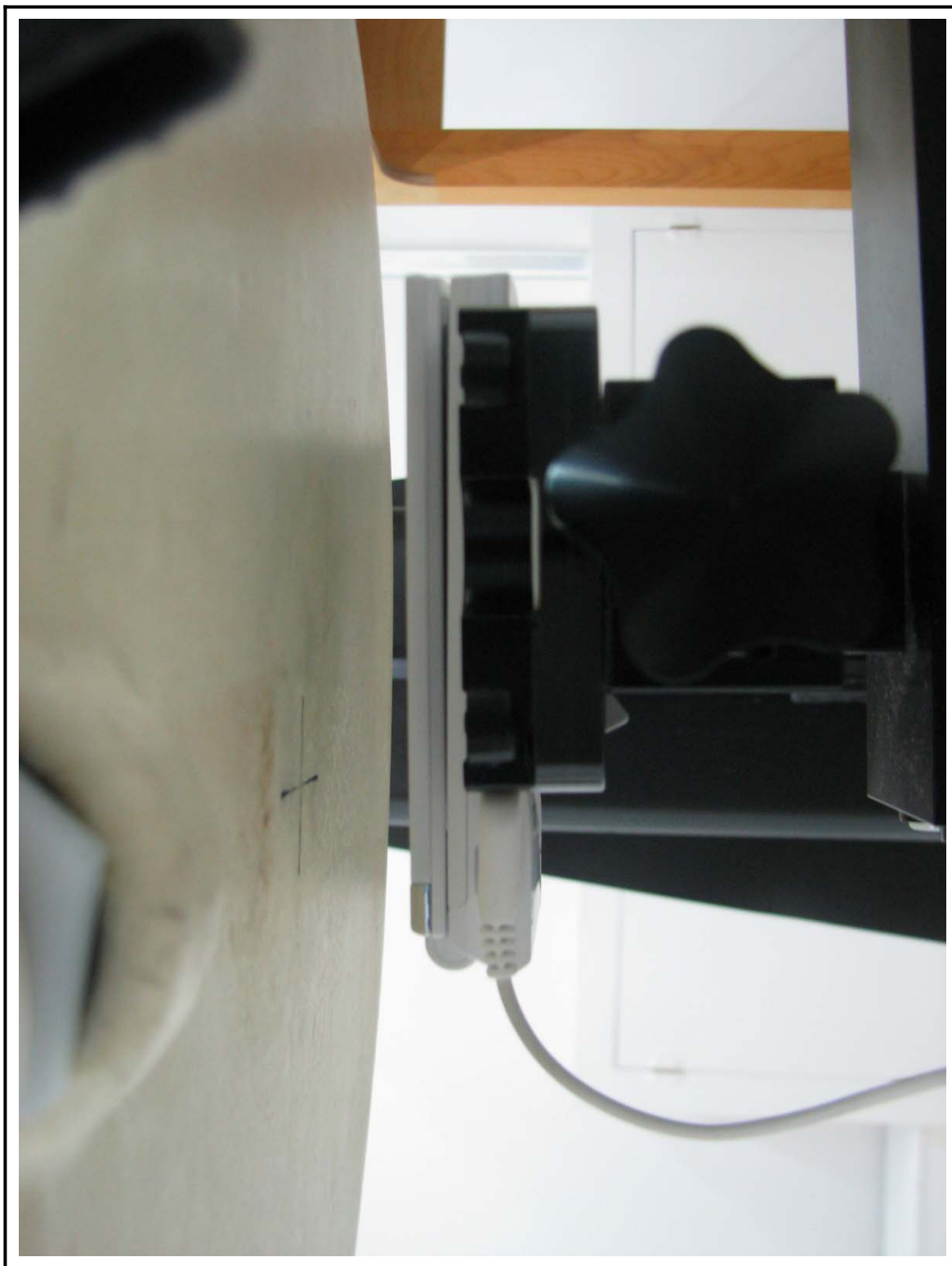
Figure 5 Body SAR Test Setup – w/o Holster
