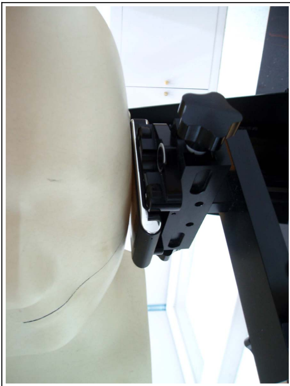
Figure 8 Left Head SAR Test Setup – Cheek Touch Position
