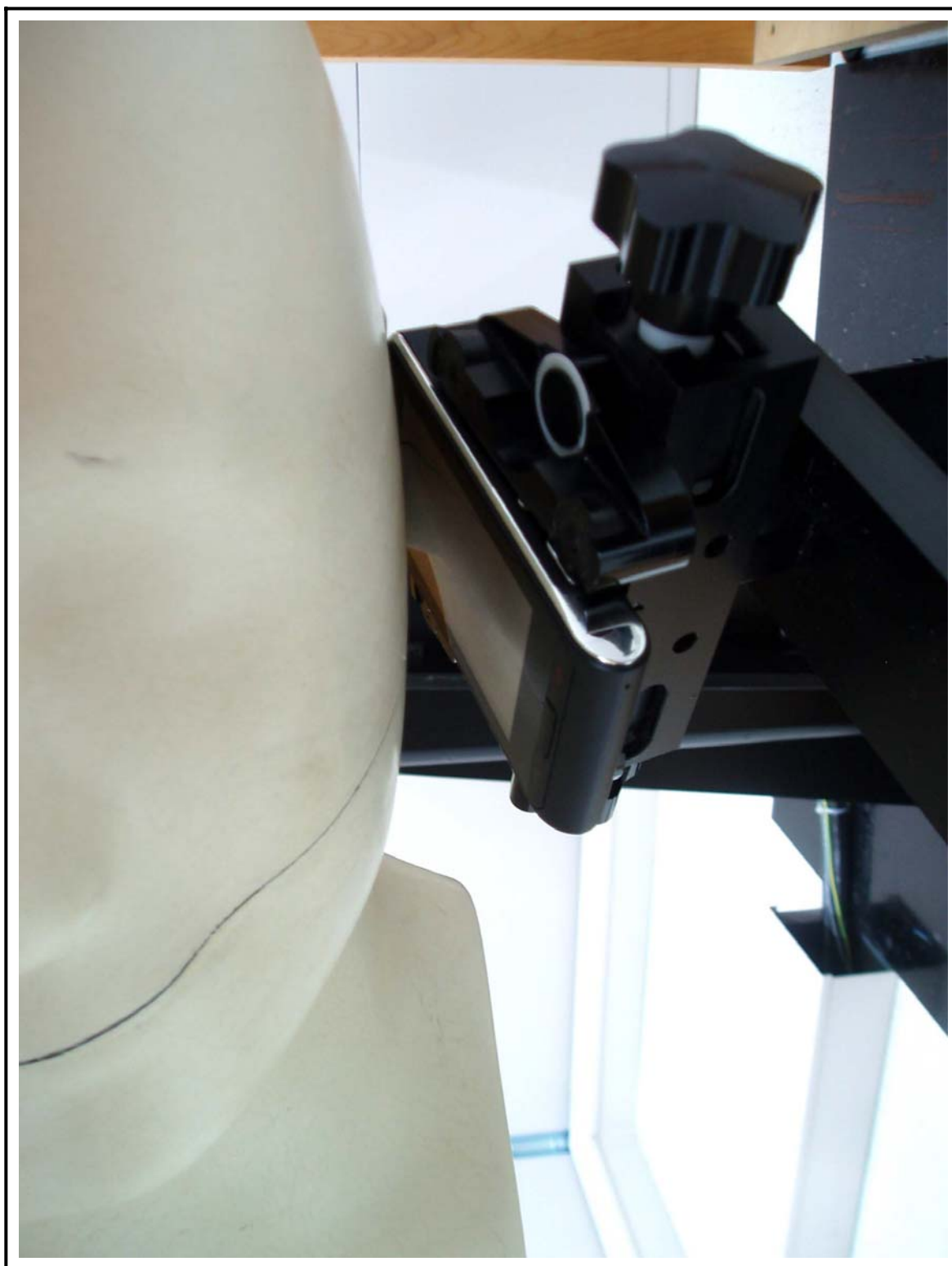
Figure 11 Left Head SAR Test Setup – Ear Tilt Position
