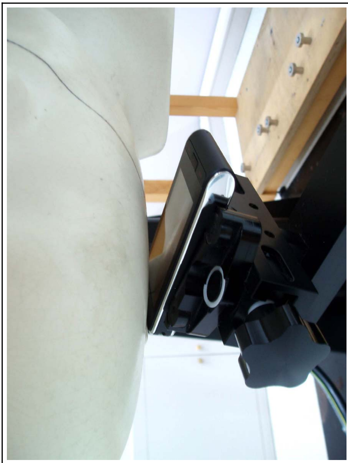
Figure 5 Right Head SAR Test Setup - Ear Tilt Position
