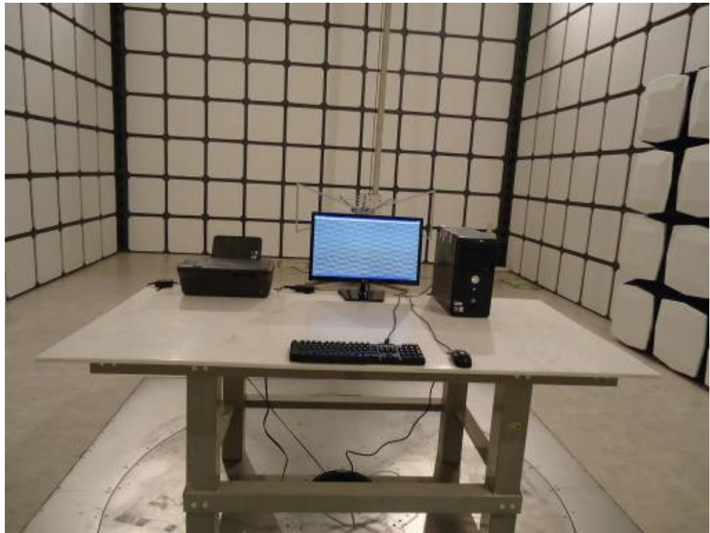
Front View of Radiated Emission Test (30MHz ~ 1000MHz)
