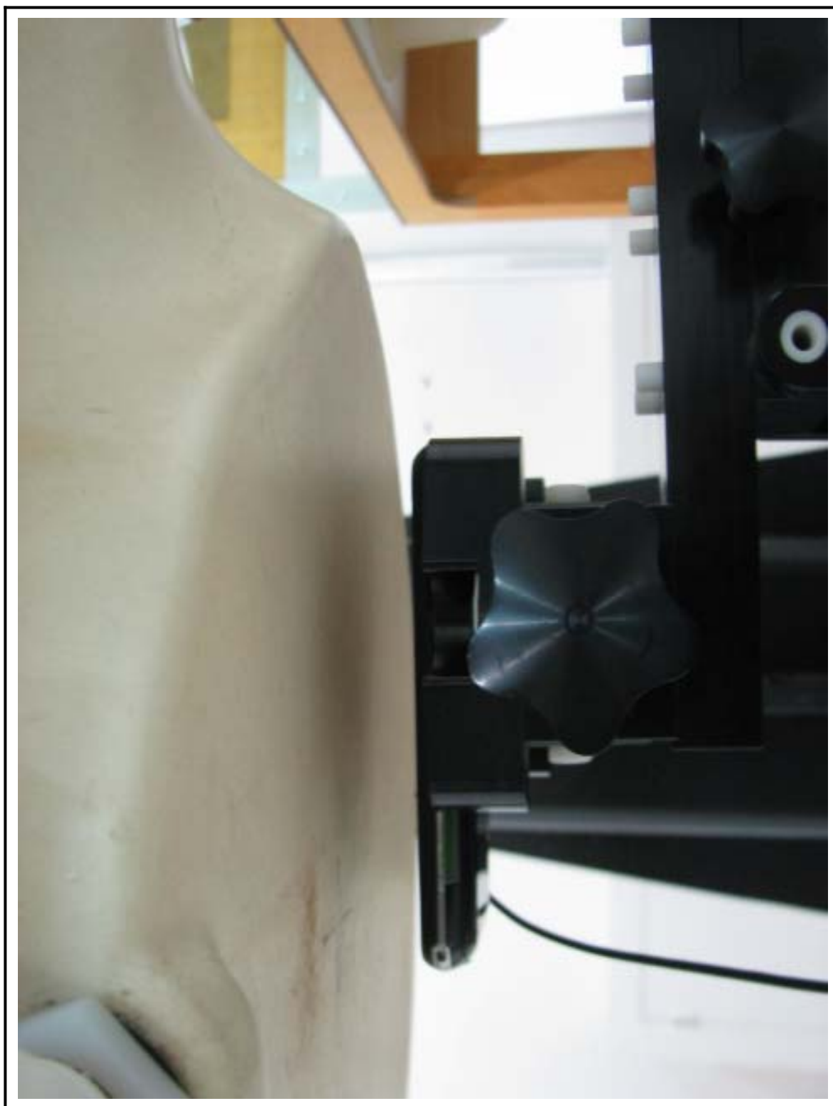
Figure 5 Body SAR Test Setup – w/o Holster
