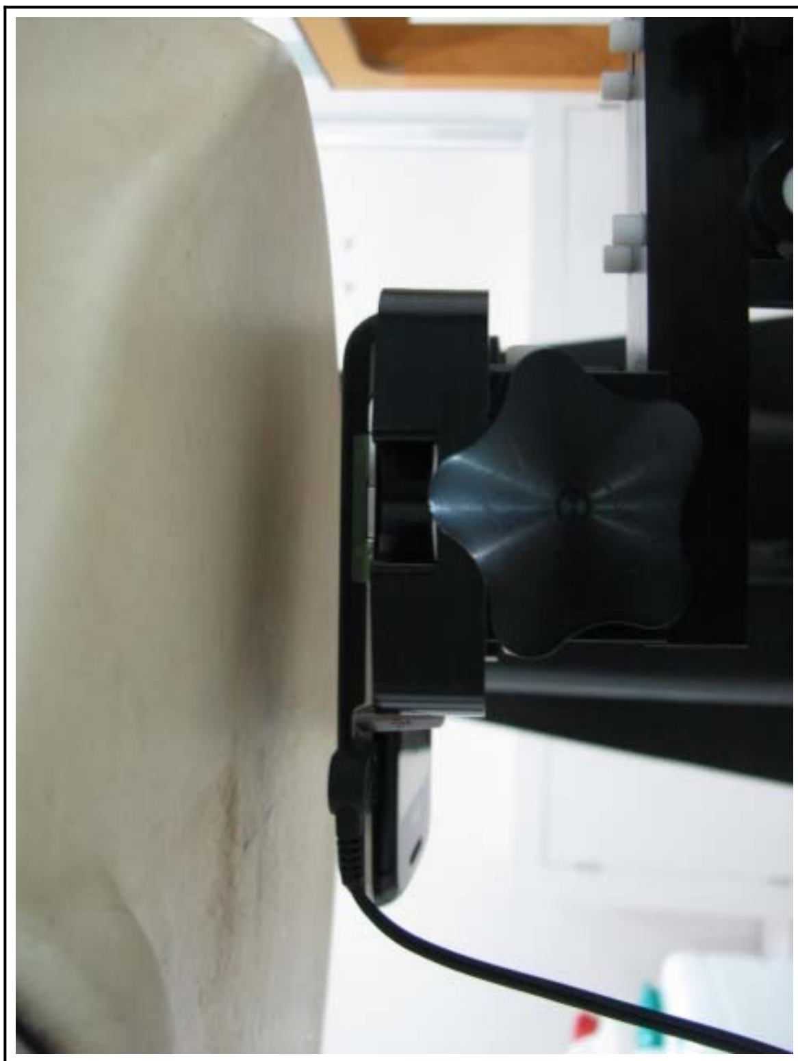
Figure 6 Body SAR Test Setup – w/o Holster
