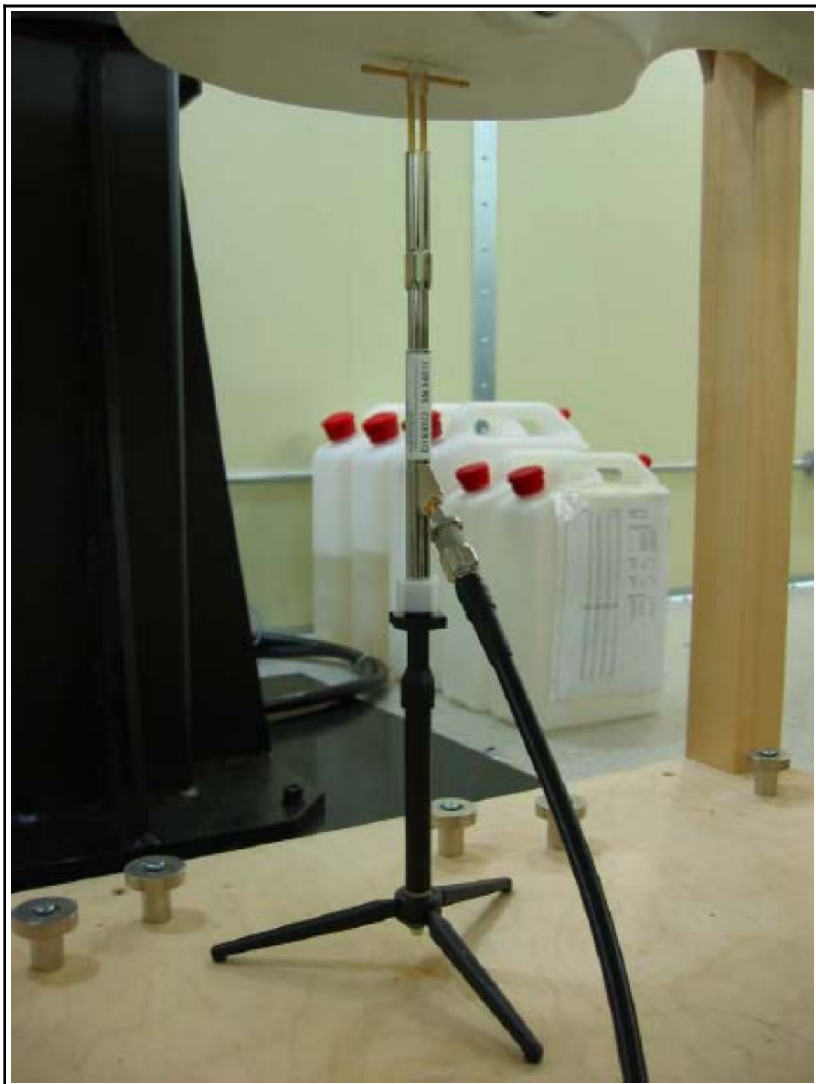
Figure 2 1900 MHz Dipole Validation Test Setup
