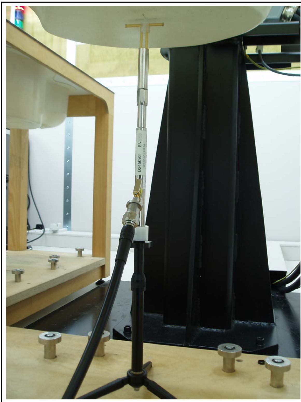
Figure 3 2450 MHz Dipole Validation Test Setup
