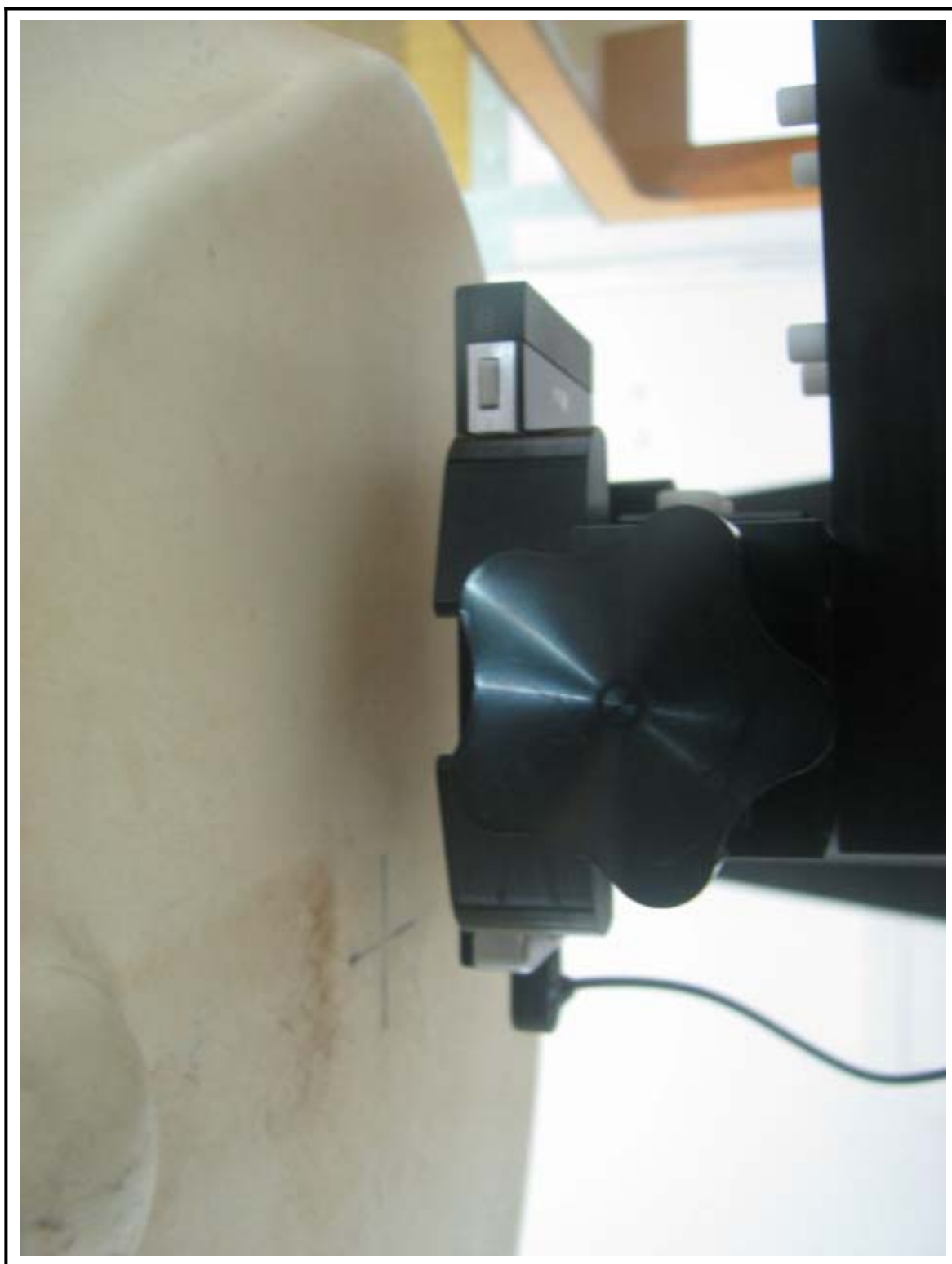
Figure 6 Body SAR Test Setup – w/o Holster
