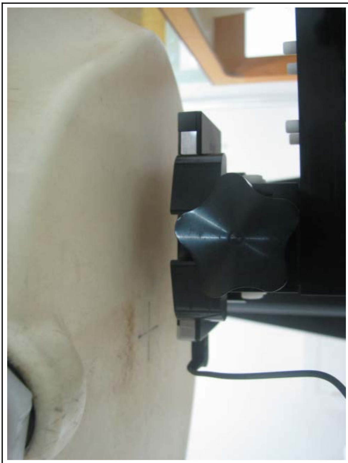
Figure 5 Body SAR Test Setup – w/o Holster
