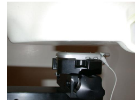
Figure 14.9 Body SAR Test Setup -- w/o Belt-clip --
