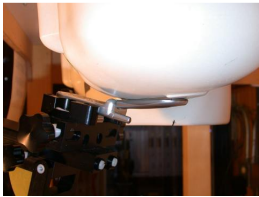
Figure 14.7 Left Head SAR Test Setup -- Cheek / Touch Position --
