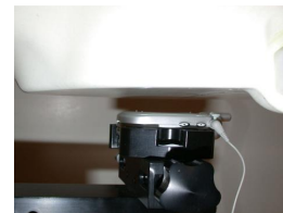
Figure 14.10 Body SAR Test Setup -- w/o Belt-clip --
