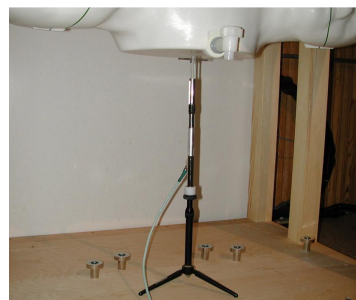
Figure 12.1 Dipole Validation Test Setup
