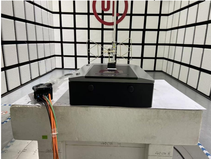
RADIATED RF MEASUREMENT SETUP (Below 30MHz)
