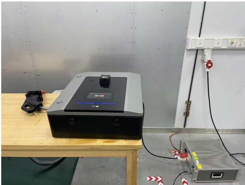
POWERLINE CONDUCTED EMISSIONS MEASUREMENT SETUP
