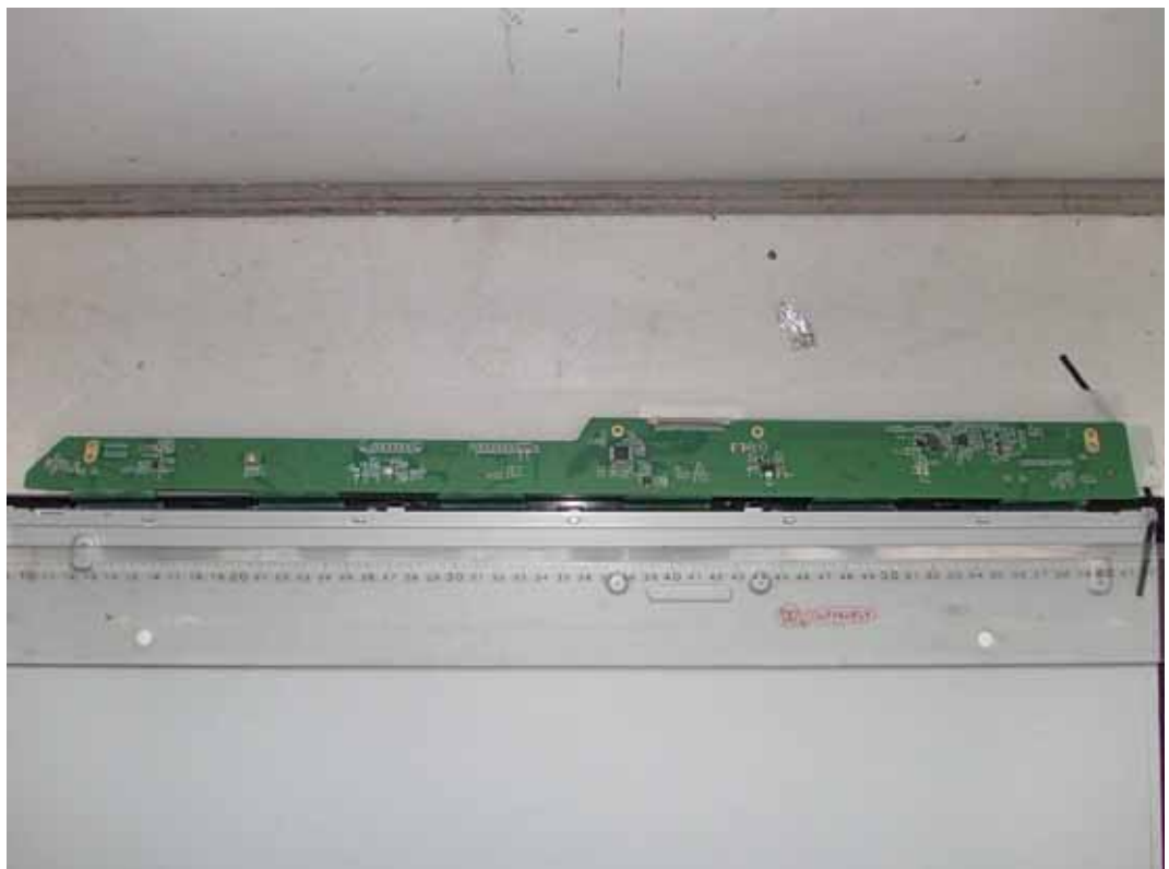
FIGURE 10 LCD MONITOR (M/N: E2442TCA) LCD PANEL BOARD (SOLDERED SIDE)
