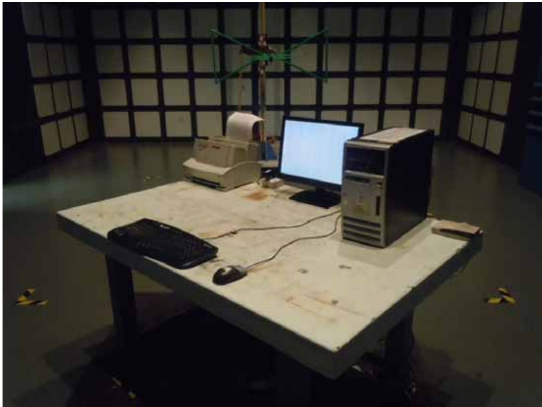
SETUP WITH MAXIMUM DETECTED EMISSION AT HORIZONTAL POLARIZATION (TEST MODE: D-SUB 1280*1024@75Hz)
