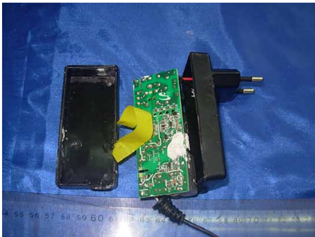
FIGURE 13 LCD MONITOR (M/N: E1948SX) ADAPTOR#2 (COVER REMOVED)
