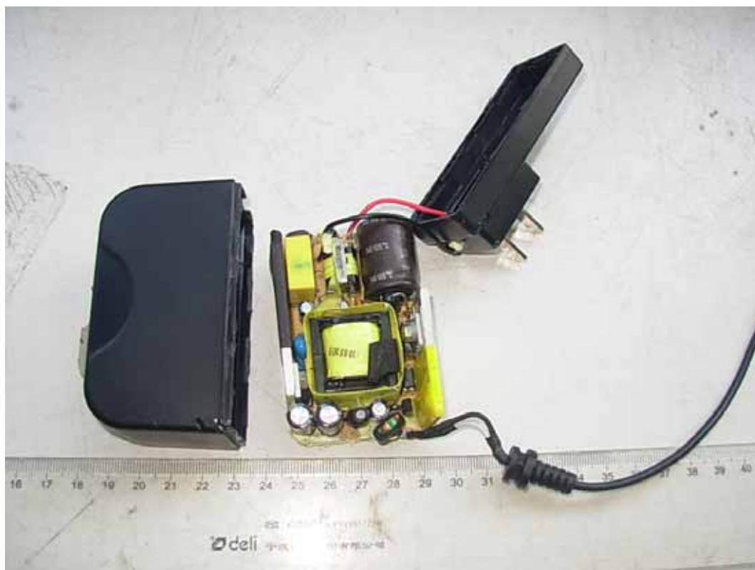
FIGURE 10 LCD MONITOR (M/N: E1948SX) ADAPTOR#1 (COVER REMOVED)
