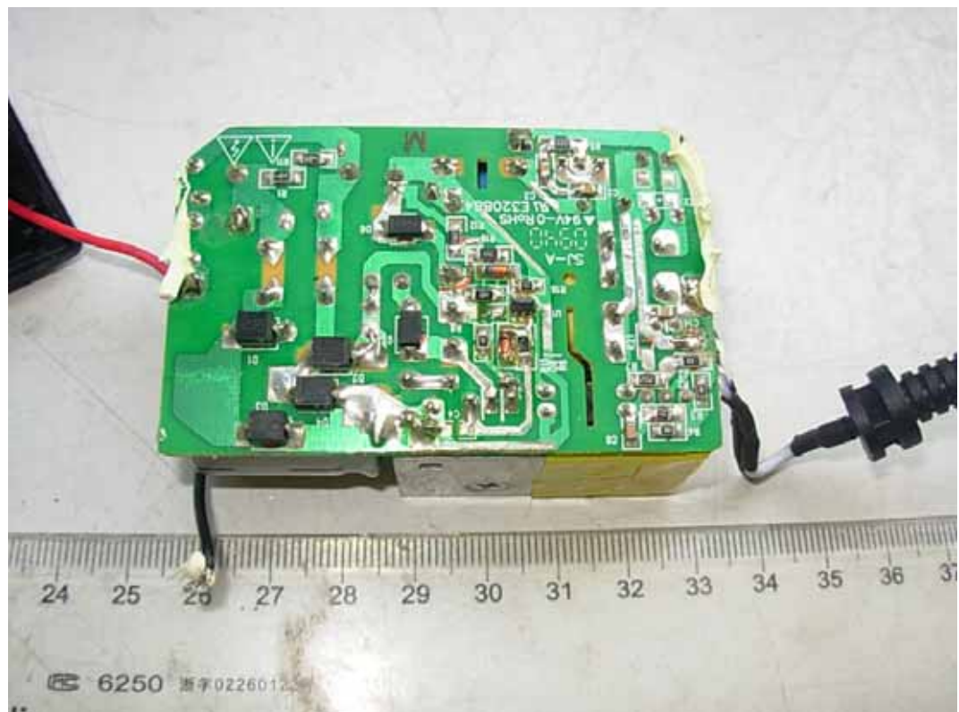
FIGURE 12 LCD MONITOR (M/N: E1948SX) ADAPTOR#1 (MAIN BOARD – SOLDERED SIDE)
