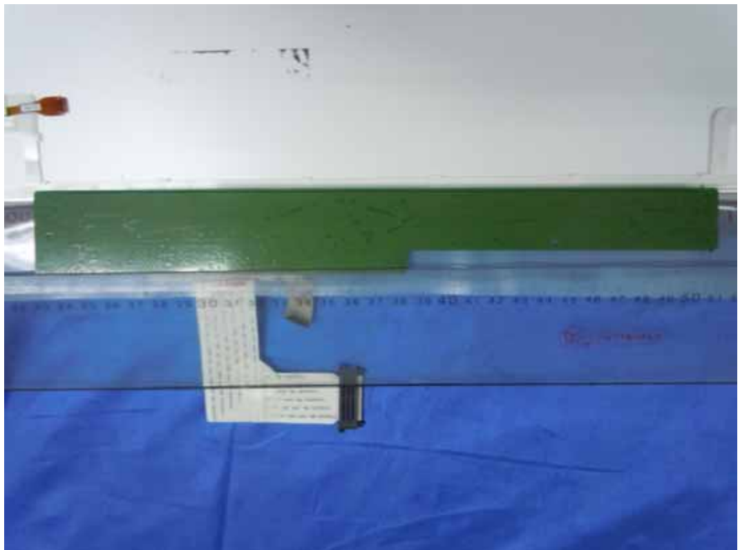
FIGURE 7 LCD MONITOR (M/N: E1642CA) LCD PANEL BOARD (SOLDERED SIDE)
