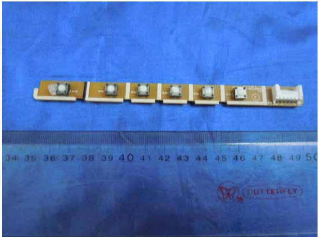
FIGURE 8 LCD MONITOR (M/N: E1642CA) KEY BOARD (COMPONENT SIDE)
