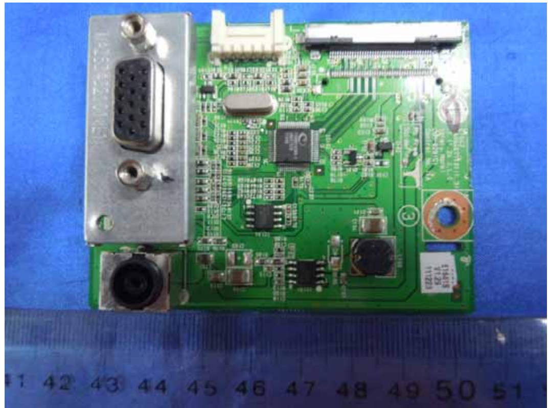
FIGURE 3 LCD MONITOR (M/N: E1642CA) MAIN BOARD (COMPONENT SIDE)
