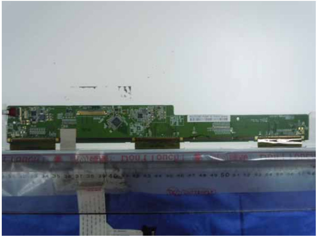
FIGURE 6 LCD MONITOR (M/N: E1642CA) LCD PANEL BOARD (COMPONENT SIDE)
