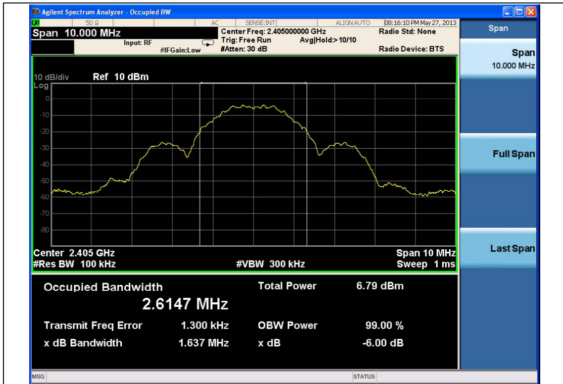
Figure 1. Plots of 6 dB Bandwidth
