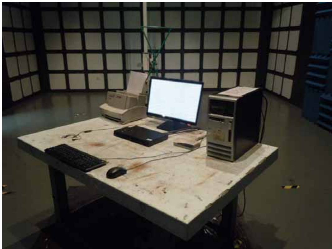
SETUP WITH MAXIMUM DETECTED EMISSION AT VERTICAL POLARIZATION (TEST MODE: D-SUB 1920*1080@60Hz Adapter #1)
