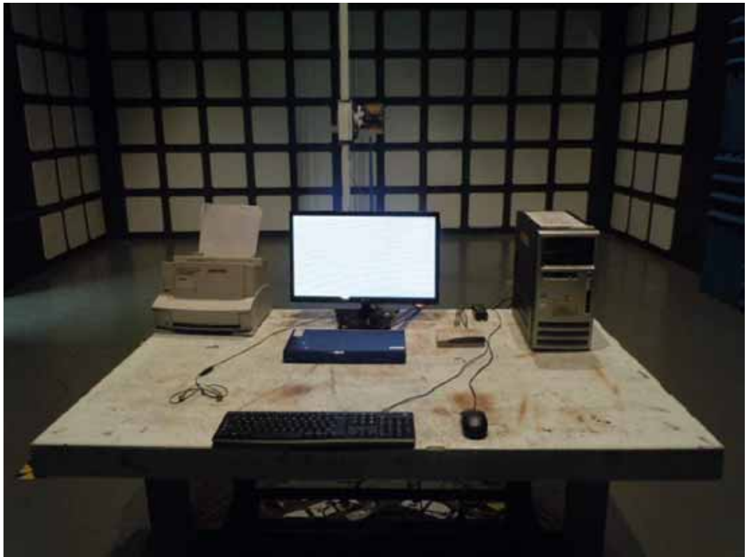
FRONT VIEW OF RADIATED EMISSION TEST (ABOVE 1GHz)
