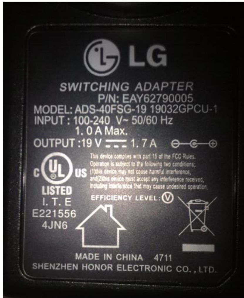
FIGURE 13 LCD MONITOR (M/N: D2343PB) ADAPTER #3 (GENERAL APPEARANCE – LABEL)
