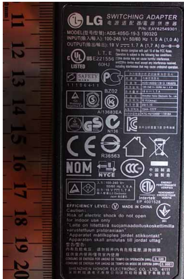
FIGURE 11 LCD MONITOR (M/N: D2343PB) ADAPTER #2 (GENERAL APPEARANCE – LABEL)
