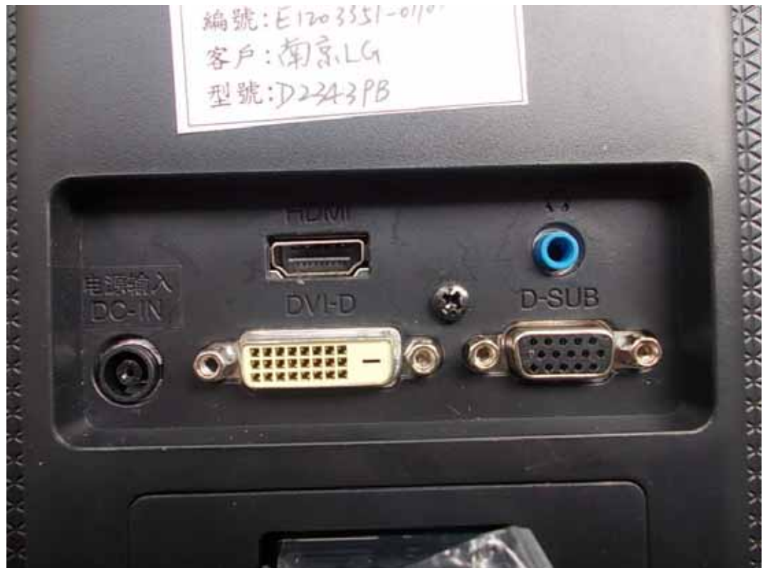
FIGURE 3 LCD MONITOR (M/N: D2343PB) PORTS
