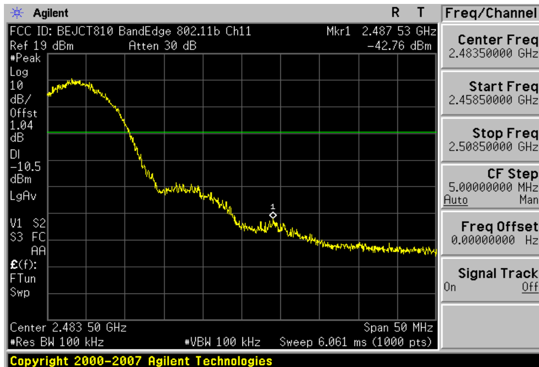
Plot 6-14. Band Edge Plot (802.11b – Ch. 11)
