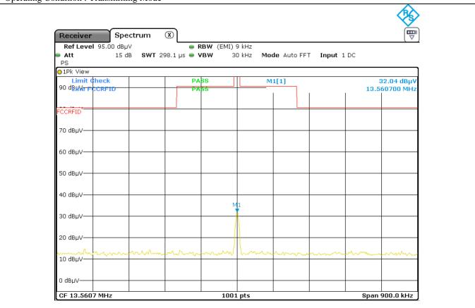
cc. to above test data, the field strength level of 13.560 7MHz is 32.04 dBuV/m and the worst limit subject to 15.225 (b) and (c) is 80.5 dBuV/m, so the EUT meets the requirement.
