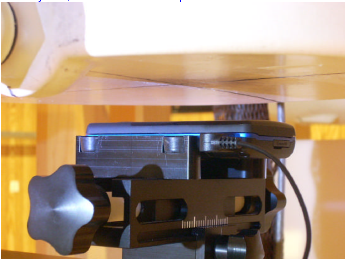
14. Body SAR, Front Side with 20mm Space
