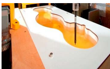
Figure 6-2 SAM Phantom with Simulating Tissue
