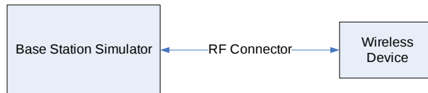
Figure 11-1 Power Measurement Setup
