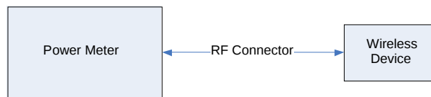
Figure 12-1 Power Measurement Setup
