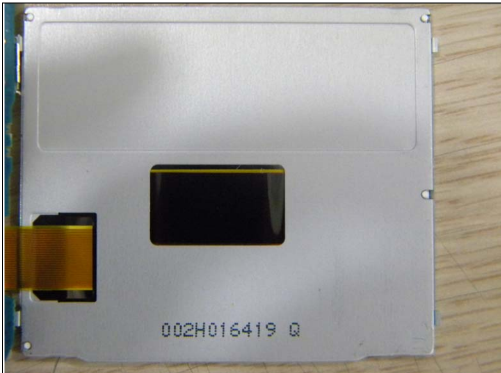
Bottom view of LCD module
