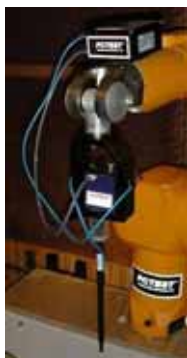
Figure 5-7 SPEAG Robotic System
