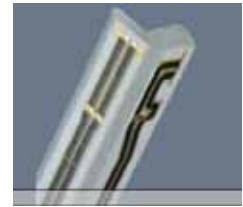
Figure 5-1 E-field Free-space Probe
