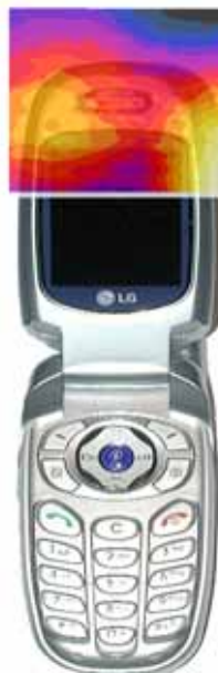
Figure 28 Sample H-field Scan Overlay
