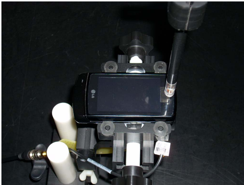
Figure 13-1 Test Setup for Wireless Device
