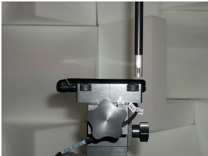
Figure 13-2 Test Setup for Wireless Device
