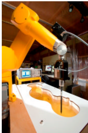
Figure 3-2 DASY4 SAR Measurement System
