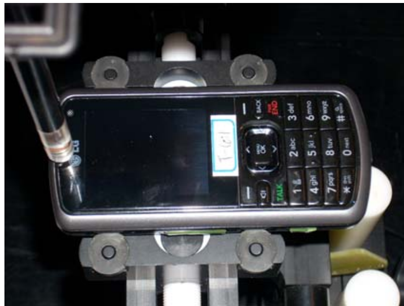
Figure 13-2 Test Setup for Wireless Device
