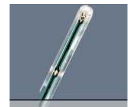
Figure 5-2 H-Field Free-space Probe
