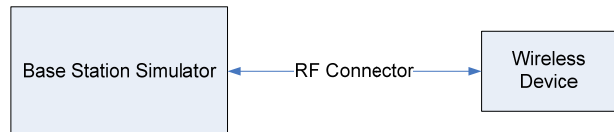
Figure 15-1 Power Measurement Setup
